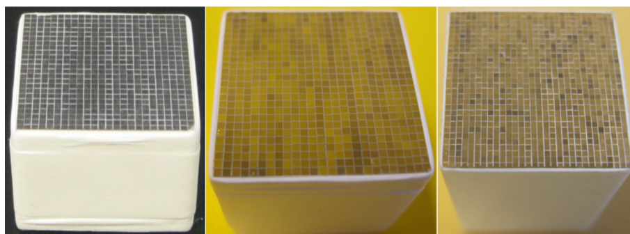
Fig. 6 LYSO arrays with different pitch sizes. (left) 1.0 mm pitch size, (middle) 0.75 mm pitch size, and (right) 0.5 mm pitch size [52, 128, 129]
