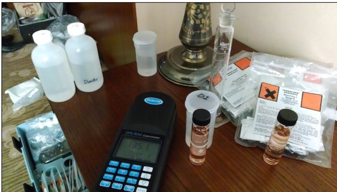
Figure 26: Analyzing village water samples with Hach CEL/850 portable laboratory (Nanning hotel room)
