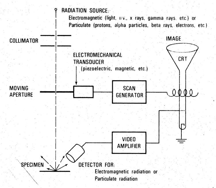
MOVING APERTURE MICROSCOPE SCHEMATIC DIAGRAM
