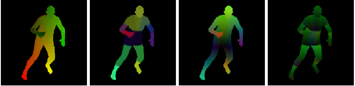
Figure 5.2: Semantic maps aligned with image space. From left to right: IUV image M_i , Dense jointmap M_j , dense location map M_l and dense displacement map M_d . (Best viewed in Color)
