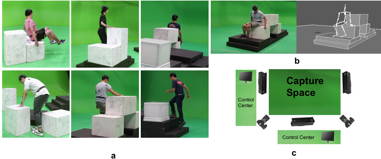
Figure 4.1: a : Samples from our data set featuring scene constrained poses: stepping on the stairs, sitting on the tables and touching boxes. b : Sample frame of a human interacting with scene geometry, and visualization of the corresponding 3D scene mesh with captured human pose. c : Motion capture setup. We simultaneously captured 3 RGBD and 2 RGB video streams and ground-truth 3D pose from a VICON marker-based mocap system. Cameras are calibrated with respect to a 3D mesh model of scene geometry.
