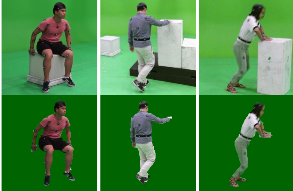
Figure 4.7: We adopt Grabcut [140] and utilize the ground truth (joints, multi-layer depth, and markers) we have to segment subjects from background. If the joints and markers are occluded by the first-layer of multi-layer depth, we set them as background, otherwise they are set as foreground in grabcut algorithm.
