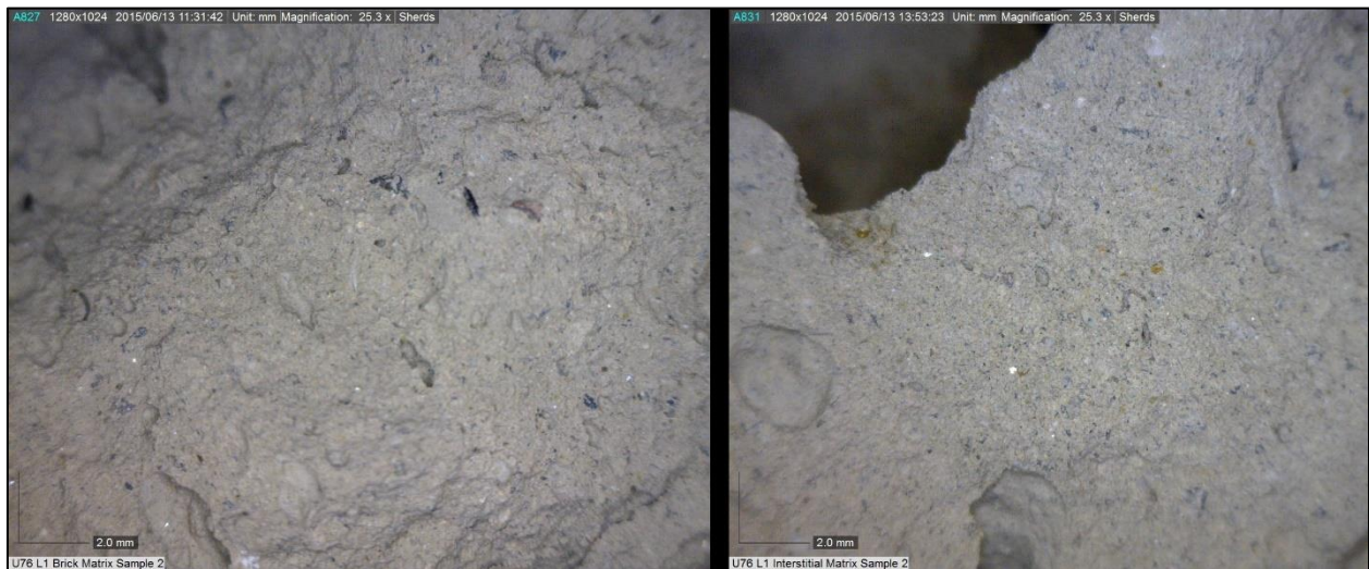
Figure 42: A comparison of cross-sections from a paraboloid adobe recovered from Huaca Soto (left) and interstitial mud-slurry matrix attached to that brick (right).
