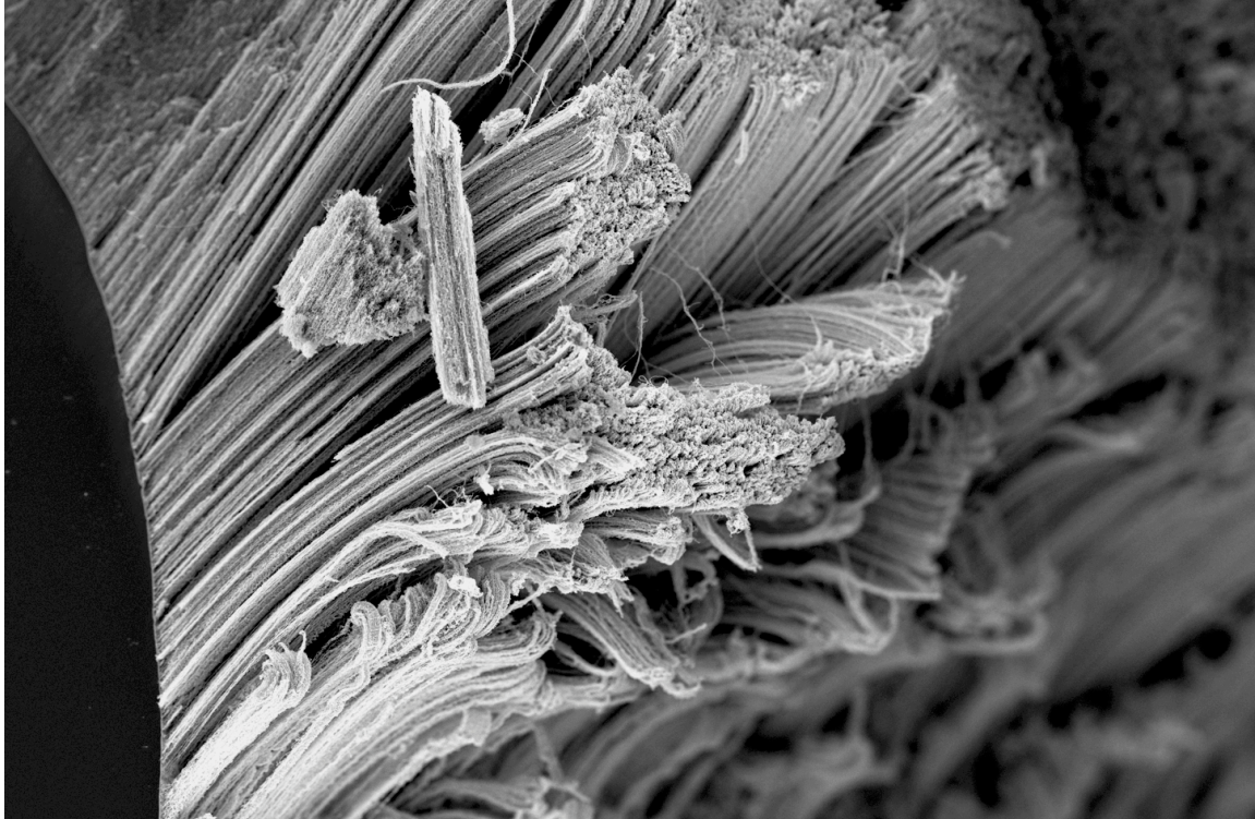
Figure 1-4: SEM image of the edge of a carbon nanotube forest. The carbon nanotubes are about 100 nm tall.
