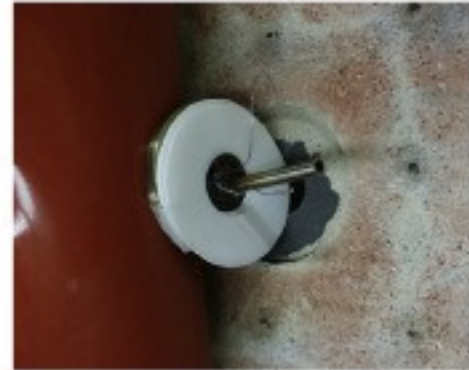
(a) Packer with inlet and outlet tubings (b) Silicone pad, packer and PTFE gasket
