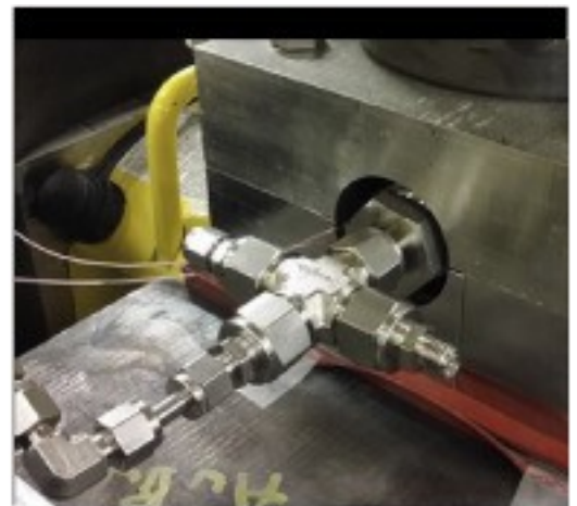
Fig. 6. Coaxial design for cryogen flow through the borehole – for unconfined specimen tests (the casing detached to show the inner inlet pipe).
