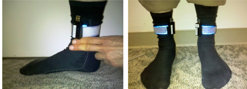
Fig 7.12 Sensor placement for SIRRACT trials
