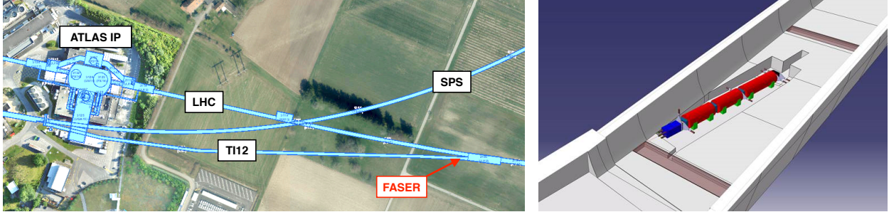
FIG. 1. Left panel: The arrow points to FASER’s location in service tunnel TI12, roughly 480 m east of the ATLAS IP. Credit: CERN Geographical Information System. Right panel: View of FASER in tunnel TI12. The trench lowers the floor by 45 cm at the front of FASER to allow FASER to be centered on the beam collision axis. Credit: CERN Site Management and Buildings Department.
