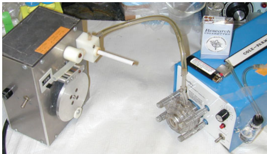
Figure 1. Example of a smoking machine that is used to create smoke solutions for in vitro testing. A peristaltic pump attached to a puffer box draws a 2 second 35 ml puff of mainstream smoke every minute. The smoke is passed through culture medium (tube to medium is not connected). The machine can also be used to make sidestream smoke solutions.
