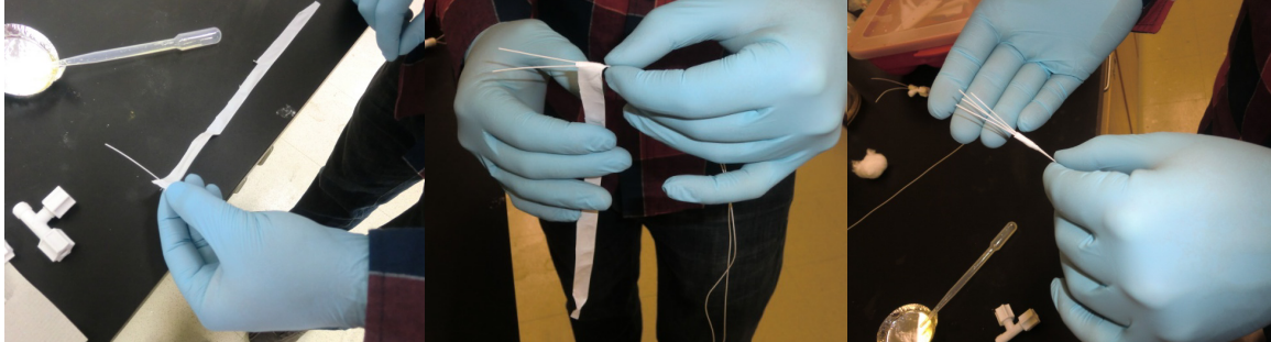
Figure F.1. Preparation of the Hollow Fiber Module. Beginning with a single fiber ( Left ), wrap Teflon tape around to hold all fibers together ( Middle ), until all fibers are taped creating the module ( Right ).
