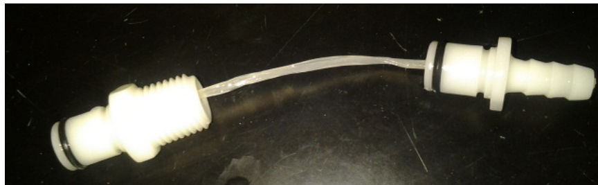
Figure F.6. Third Generation Osmotic Transport Device. Hydrogel not shown.
