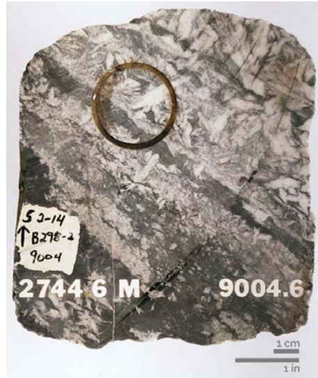
Figure A4.10. Interbedded mudstone and anhydrite from 2744.6 m (9004.6 ft) depth in the State 2-14 drill core.
