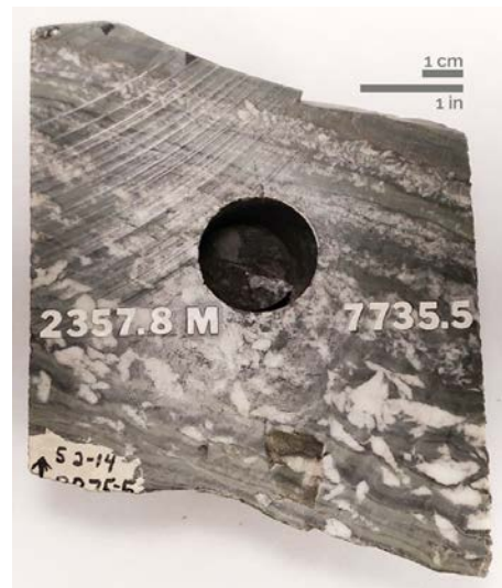
Figure A4.8. Interbedded mudstone and anhydrite from 2357.8 m (7735.5 ft) depth in the State 2-14 drill core.
