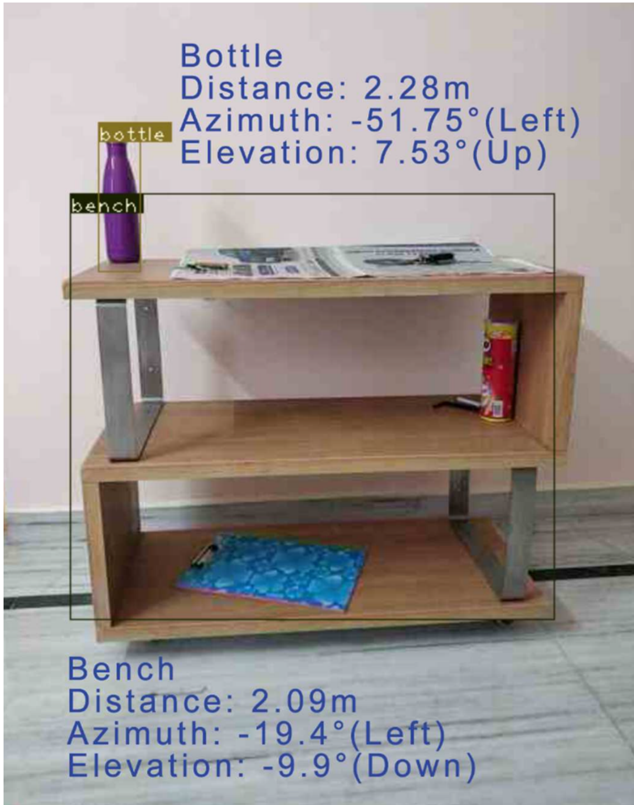
Figure 4.1: Example of indoor navigation system with distance
