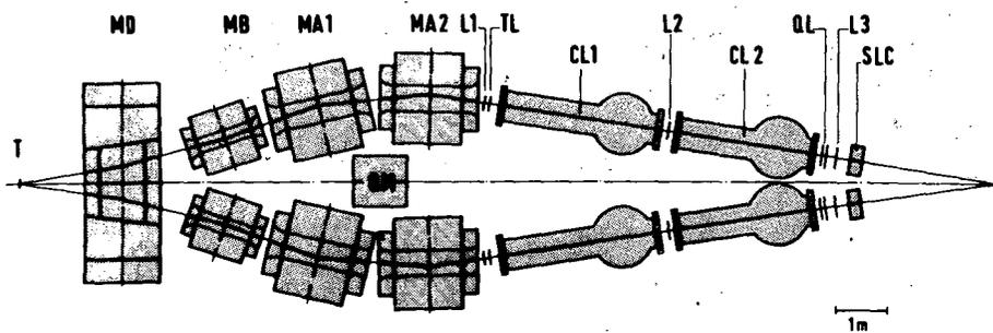
Fig. 1. The DESY-MIT double-arm spectrometer.
