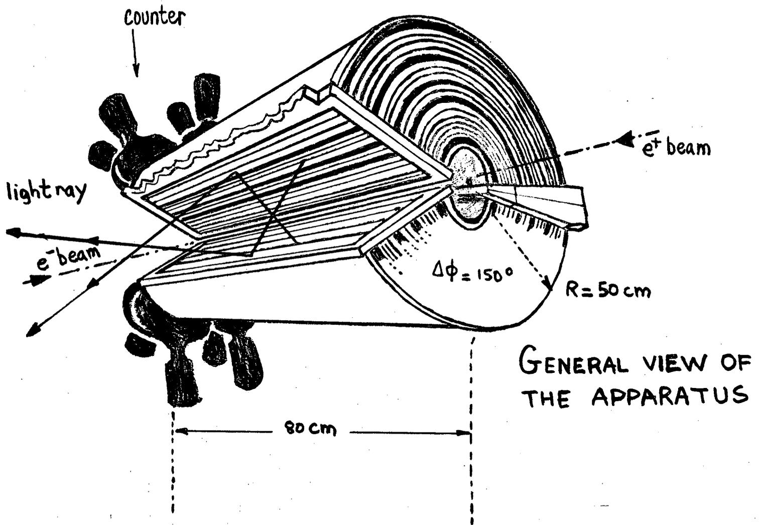
Fig. 5a. Sketch of cylindrical spark chamber arrangement used in the Orsay experiment.
