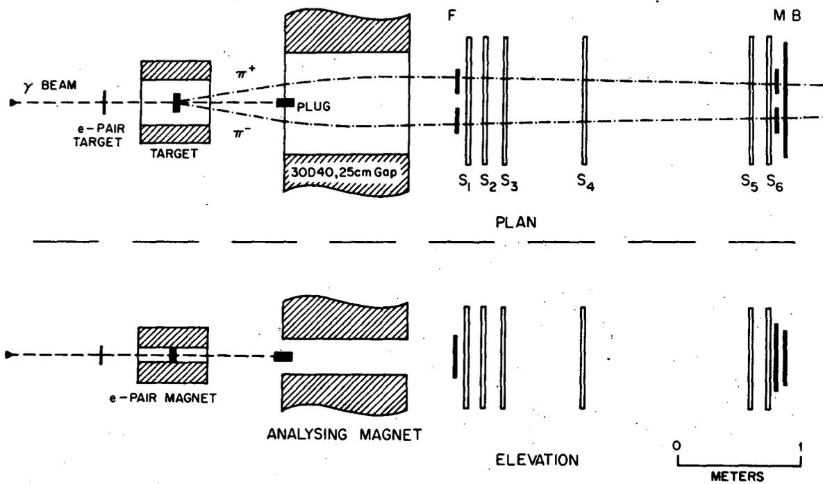
Fig. 3. Plan and elevation views of the experimental layout of the Rochester-Cornell-NAL group.
