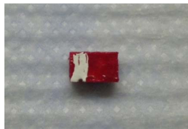
Figure 3 White marking indicating etched half of unetched – etched sample.
