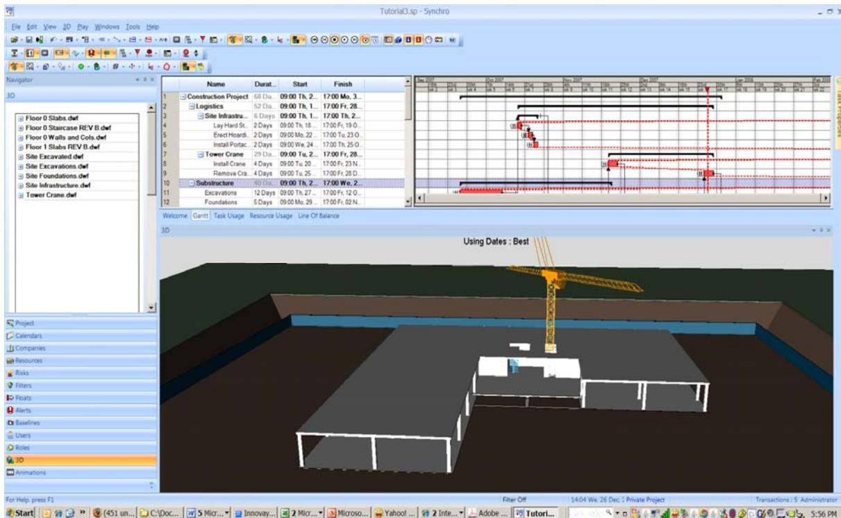
Figure 3.4 4D scheduling using Synchro
