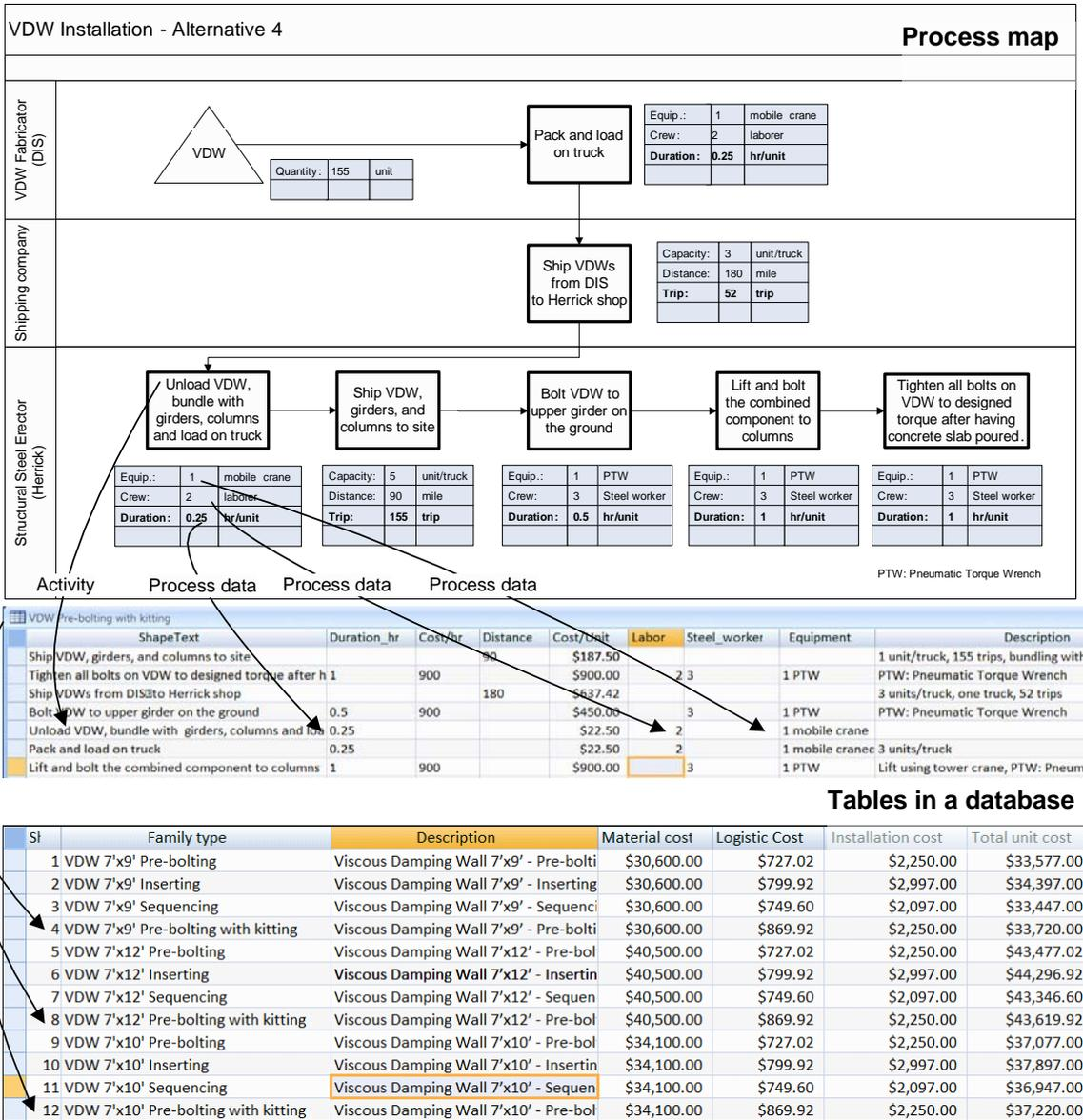
Figure 4.7 Data inputted from a process map to a database
