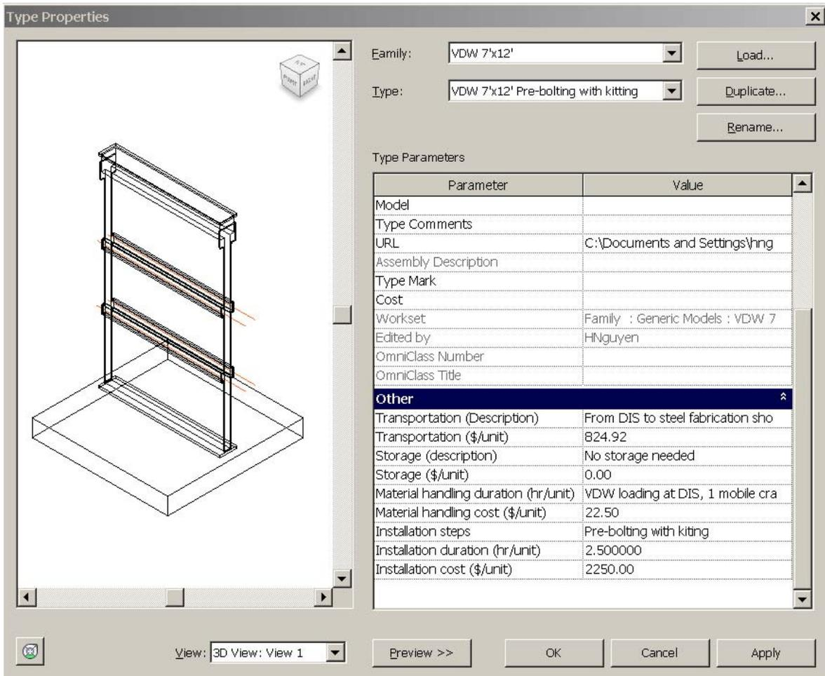
Figure 7.16 Connect detailed process- and cost data to an object family type
