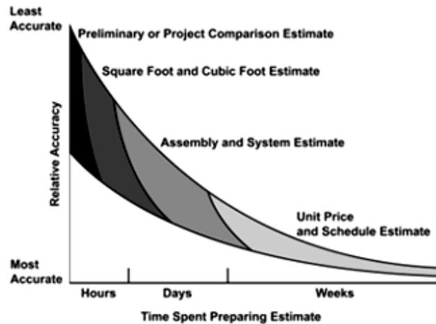
Figure 3.2 Relative accuracy of estimate types (Bledsoe 1992)
