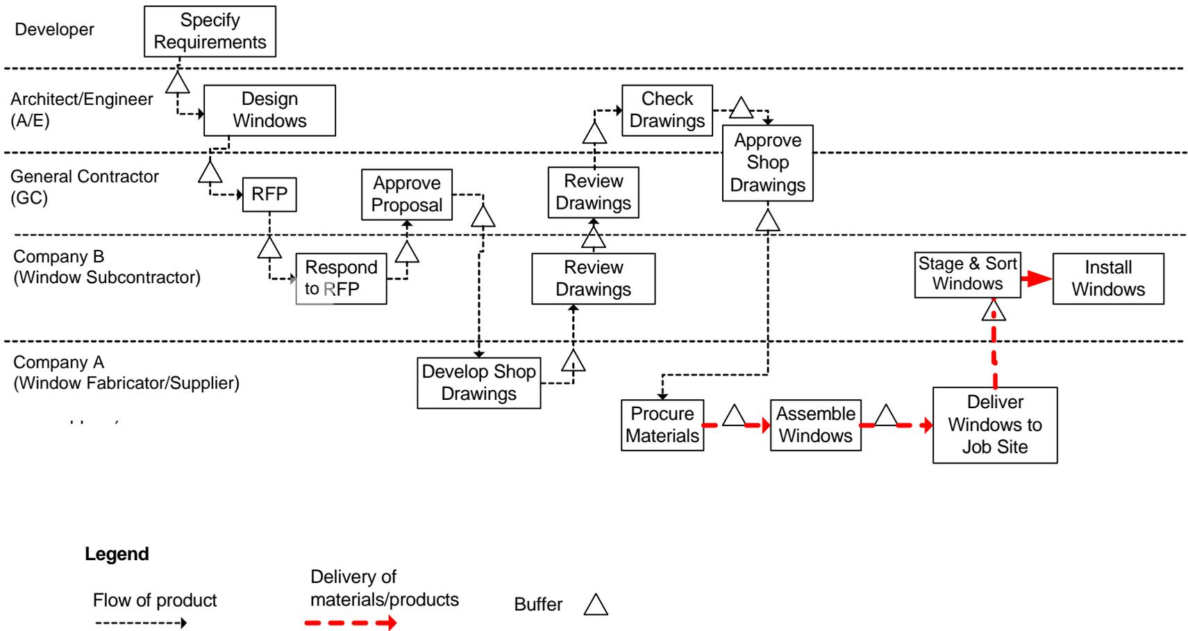
Figure 5.5 Cross-functional process map of window supply chain activities in Project X
