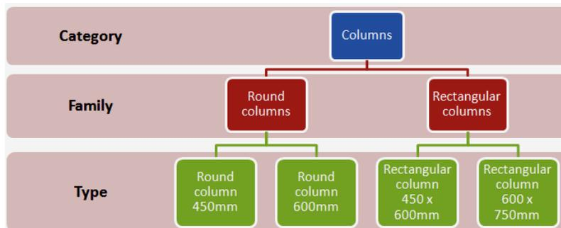
Figure D.1 Element classification structure in Revit Architecture (Autodesk 2009a)
