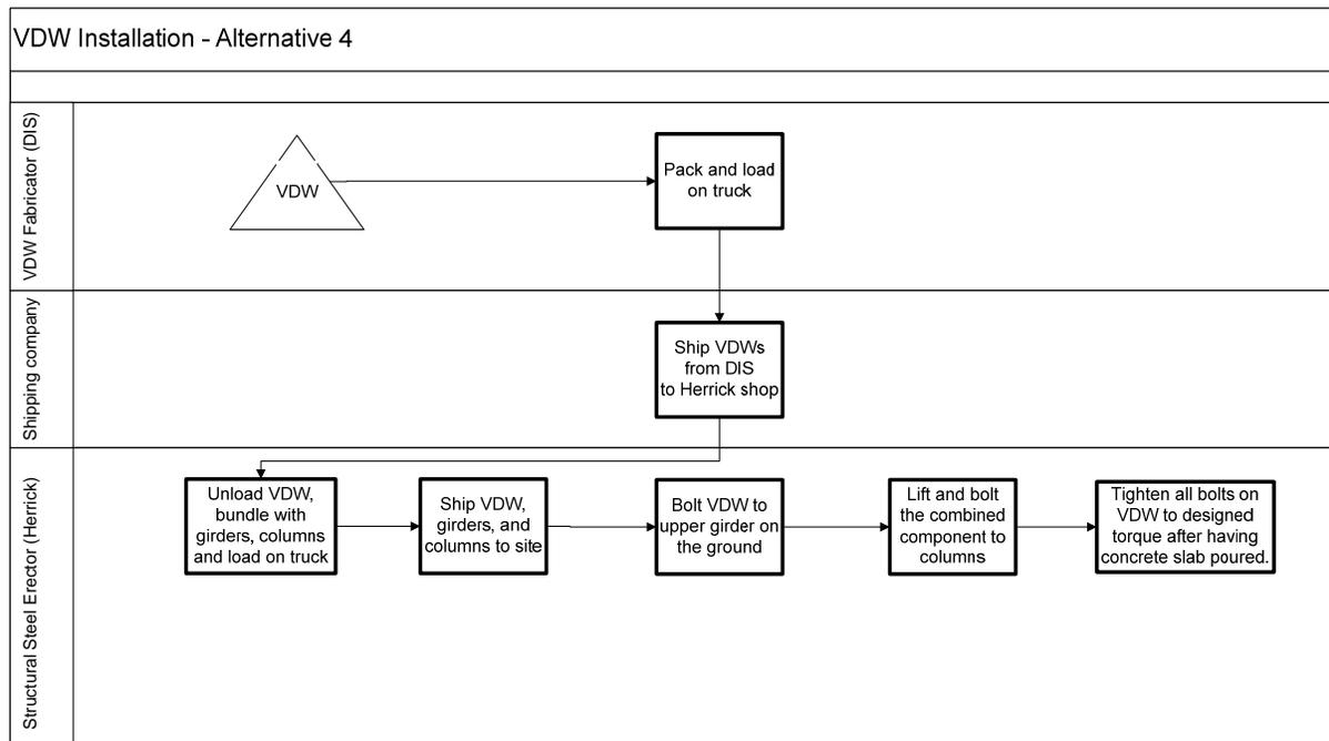
Figure 6.9 Cross-functional process map of installation alternative 4
