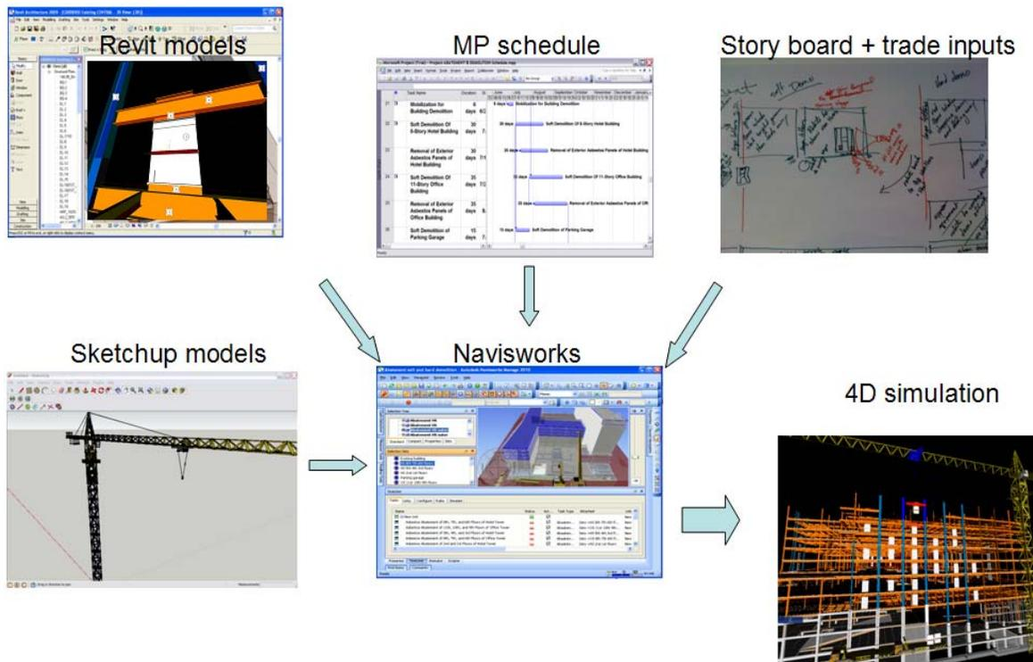
Figure 6.4 Inputs to 4D simulation
