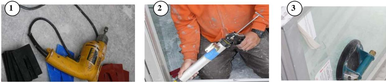
Figure 5.8 Hand tools for window installation
