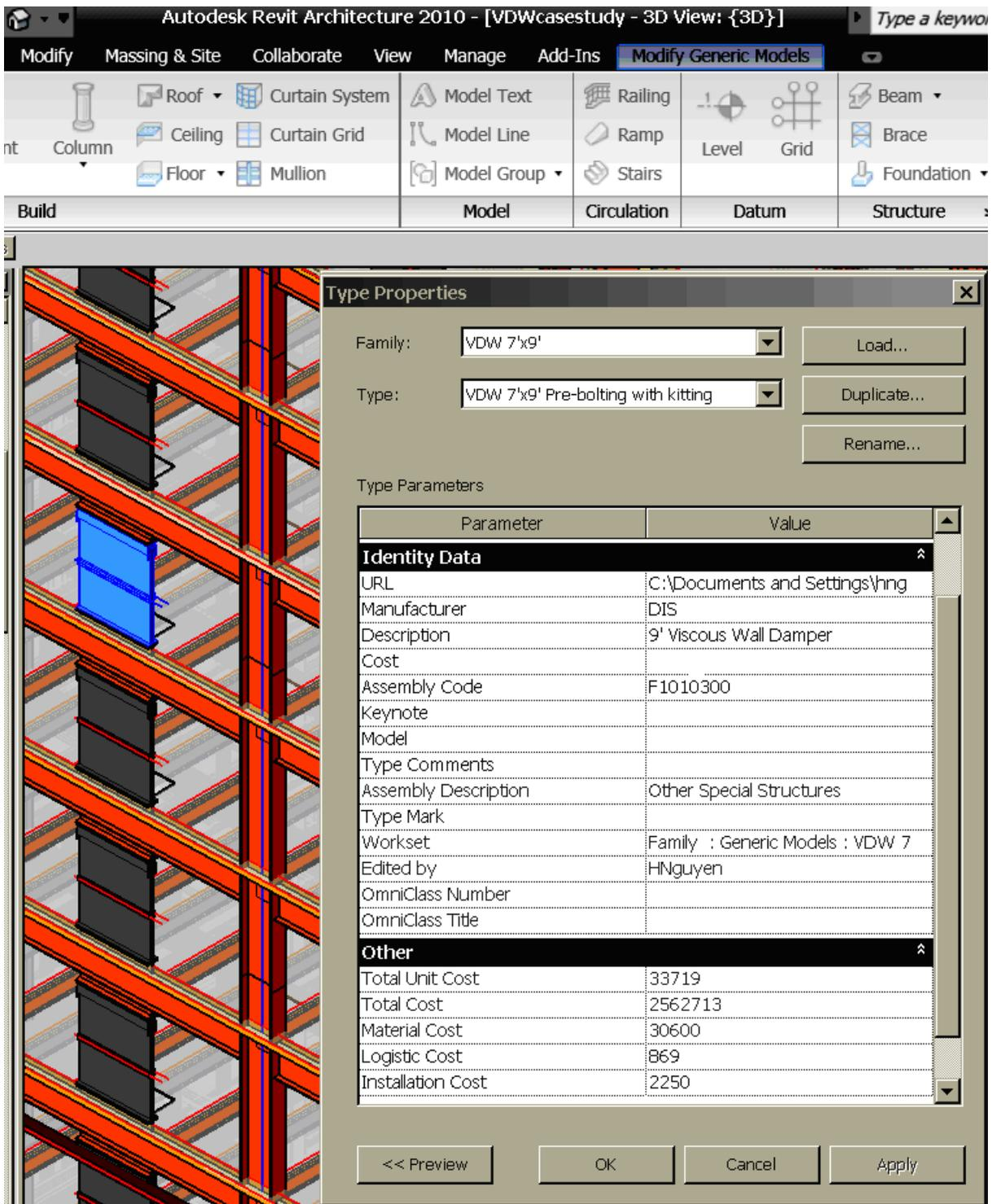
Figure 7.10 Cost data is linked to BIM object and displayed on the object property list
