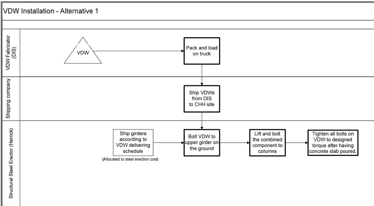
Figure 6.6 Cross-functional process map of installation alternative 1
