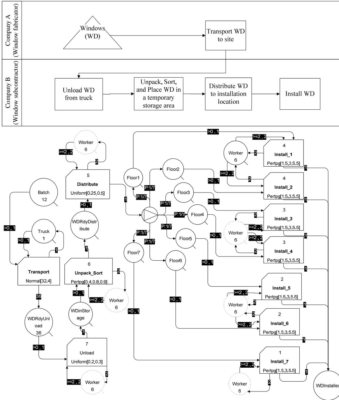
Figure 5.19 Current state map and current state simulation model of window site handling and installation processes
