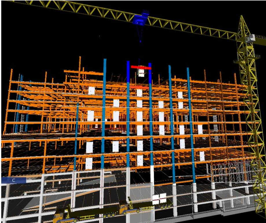
Figure 6.5 Frame in the 4D simulation of the VDW installation alternative 1
