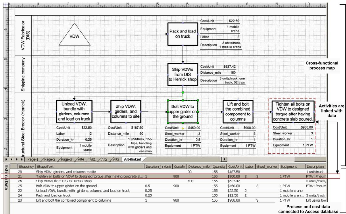
Figure 7.4 Shapes in a process map in Microsoft Visio 2007 link to process- and cost data in Microsoft Access 2007 using ODBC
