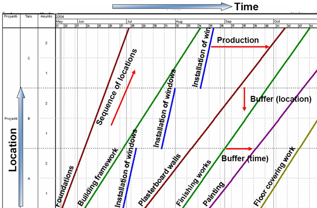
Figure A.2 Example of a location-based schedule (courtesy of Vico)
