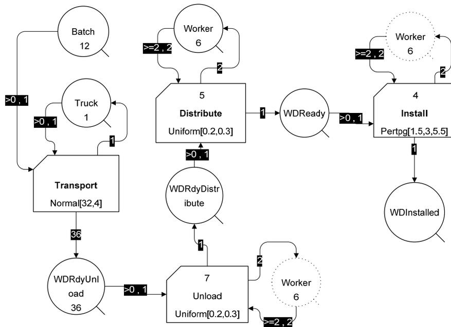
Figure 5.20 Future state process map and simulation model of window site handling and installation processes
