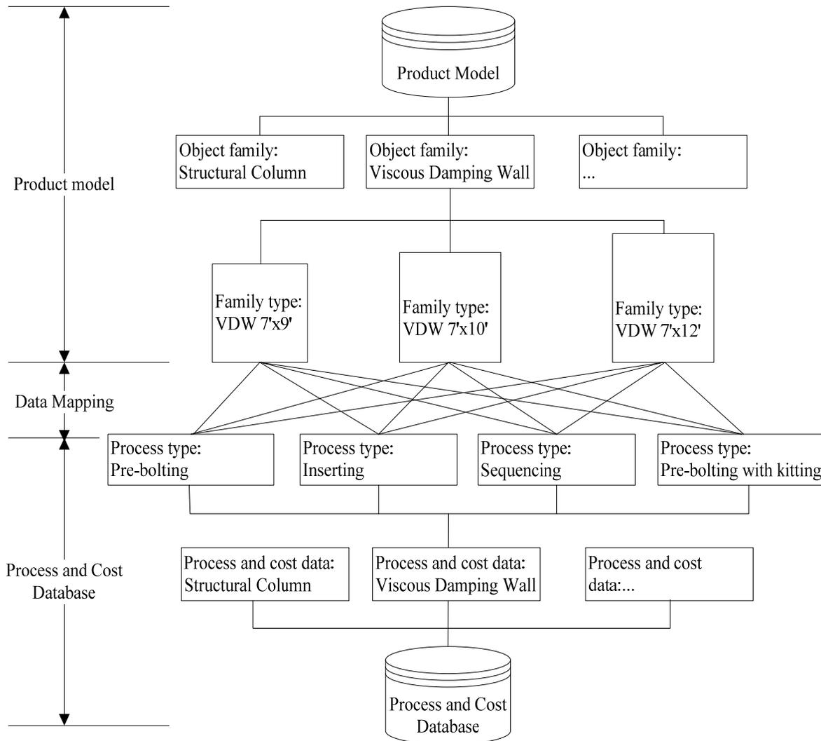
Figure 4.8 Linking object family types of a product model to process cost data
