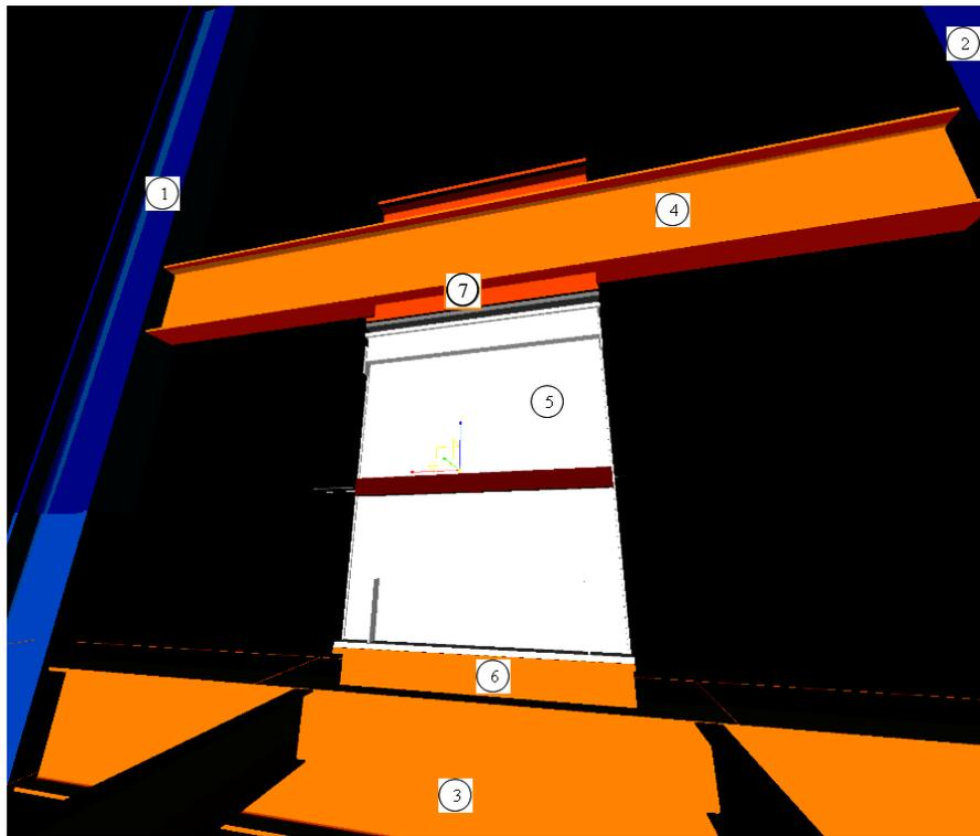
Figure 6.2 3D rendering of a VDW attached to structural steel
