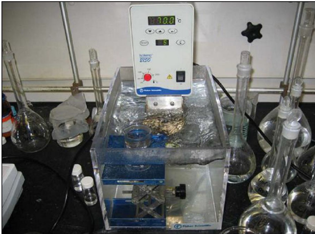
Figure 1.2.5 – Water bath setup for PET cylindrical pore etch. 0.5M NaOH solution at 70° C is used. The damage track is etched at a rate of 1200 nm / minute and the bulk polymer at 1.67 nm/ minute under these conditions.
