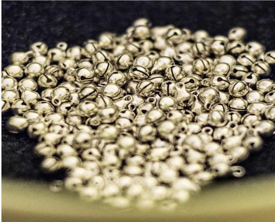
Figure 9. 6mm jingle bells in foam-covered ceramic bowl that allowed for the reproduction of time-varying pitch and timbral profiles as exhibited by electronic tinnitus models.
