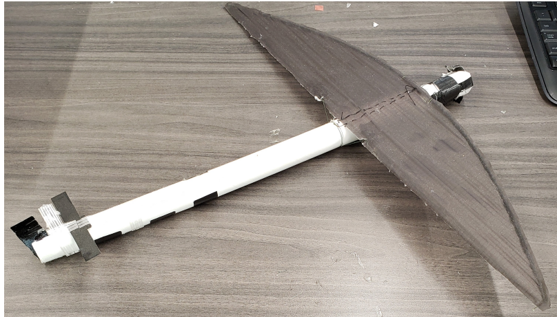
Figure 2.2: Rip-Stop Nylon Wing Glider
