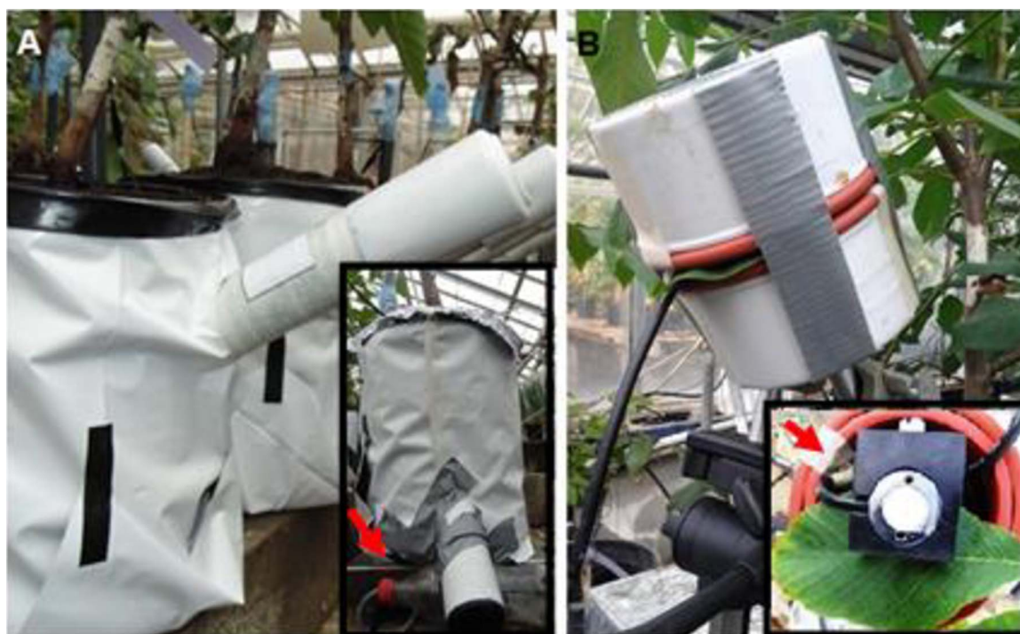
Fig. 1. Pots equipped with minirhizotrons tubes, on the weighing scales with the tensiometer and plastic reservoirs to collect the leached water (A); and a leaflet equipped with the psychrometer and the insulation capsule (B) Photo: Daniela Jerszurki.
