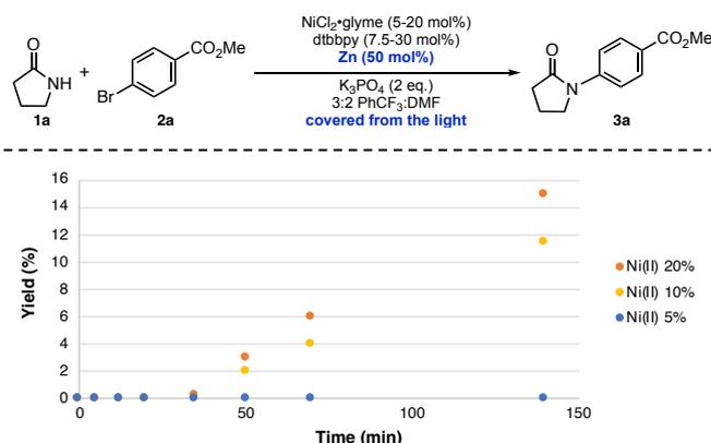
Figure 7. Effect of Ni concentration on reaction rate utilizing Zn as chemical reductant in the absence of photocatalyst and light. Reaction conditions: NiCl<sub>2</sub>·glyme (0.01 mmol to 0.04 mmol), dtbbpy (0.015 to 0.06 mmol), Zn (0.1 mmol), K<sub>3</sub>PO<sub>4</sub> (0.4 mmol), aryl bromide **2a** (0.2 mmol), amide **1a** (0.4 mmol), 0.50 mL DMF, and 0.75 mL of PhCF<sub>3</sub>. All yields were determined by <sup>1</sup>H NMR analysis.
