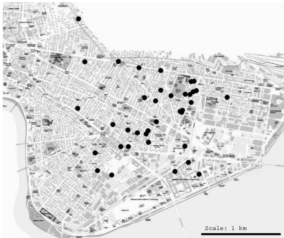
Figure 3.1: The Roofnet mesh network. Reproduced from [ABB + 04].
