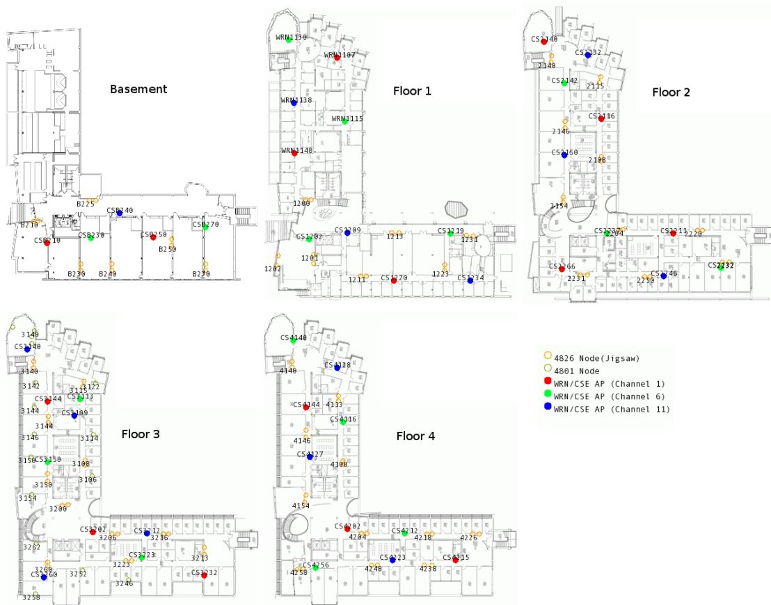
Figure 3.2: The UC San Diego Jigsaw wireless testbed. For our work, we use the Jigsaw mesh nodes (depicted as circles); production 802.11 access in the building is provided by traditional infrastructure-mode access points (represented as triangles).
