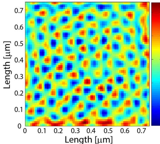
**Figure 3.** STXM image taken at the absorption peak in the O K edge for a  $\text{PS}_{124}\text{P2VP}_{61}$  sample after PSS deposition. Blue indicates strong absorption, i.e. higher oxygen content.
