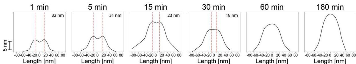
**Figure 5.** Averaged cross-sections through the centers of 18 wide cylinders, taken after different incubation times in PSS solution. The widths of the gaps marked by the vertical dashed lines are provided in the top right corner. Scale bar refers to the y-axis.
