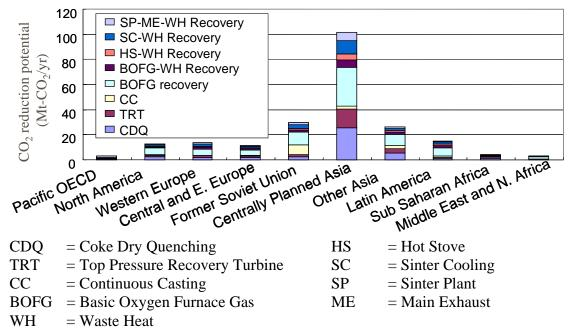
15 Figure 7.1: CO<sub>2</sub> reduction potential of eight energy saving technologies in 2030 Note: B2 Scenario, CO<sub>2</sub> emission reduction based on energy saving assuming 100% diffusion in 2030 less current diffusion rates.
