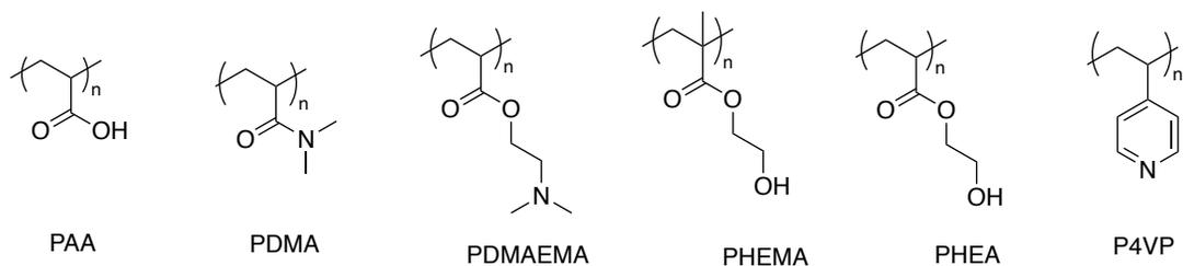
Figure 1.13: Structure of polymers grafted from the surfaces of PVC sheets and tubing<sup>64</sup>
