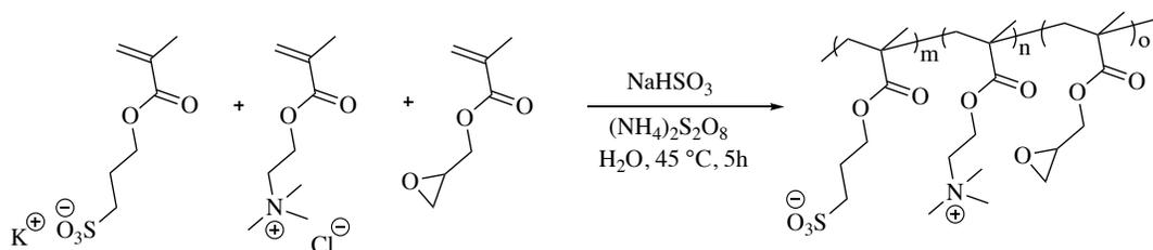
Figure 1.7: Random co-polymerization to form zwitterionic PSTG<sup>50</sup>
