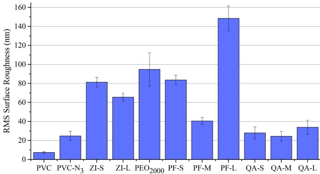
Figure 2.13: Root mean square roughness of modified PVC tubing
