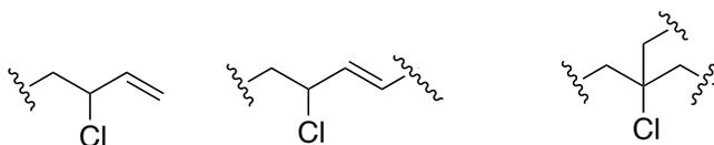
Figure 1.15: Structural defects present in PVC
