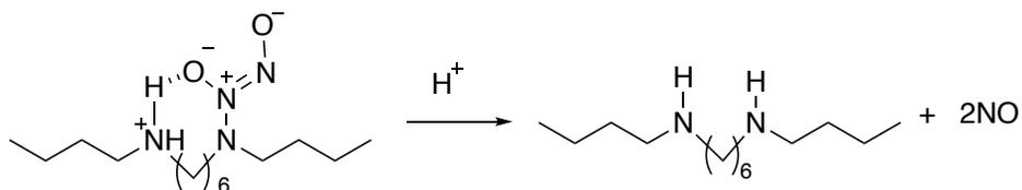
Figure 1.25: Diazoniumdiolated dibutylhexanediamine releases NO<sup>123</sup>
