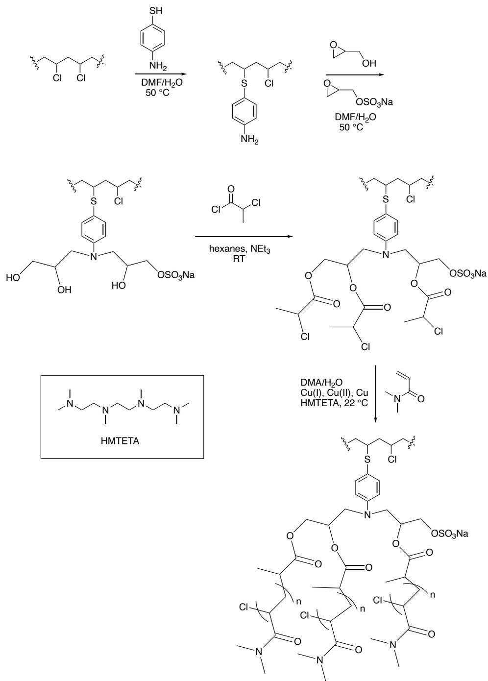
Figure 1.16: Addition of an ATRP initiator onto PVC followed by SI-ATRP<sup>67</sup>
