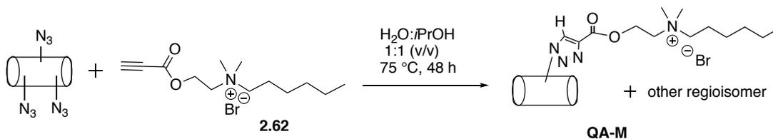
**PVC surface modified by 2-propynoic acid, 5-*N*-hexyl-*N*-ethyl-*N,N*-dimethylammonium bromide ester (2.62) (QA-M)**
