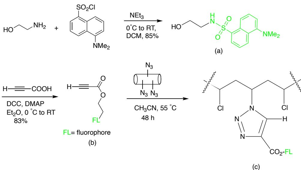
Figure 2.6: Fluorophore attachment on PVC tubing by thermal azide-alkyne cycloaddition
