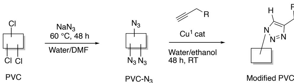
Figure 1.10: PVC surface modification with polysaccharides and PEG functional groups by Cu mediated azide alkyne cycloaddition<sup>59</sup>
