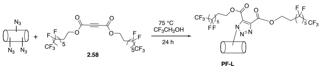
**PVC surface modified by 2-butynedioic acid, 1,5-bis(3,3,4,4,5,5,6,6,7,7,8,8,8-tridecafluorooctyl) ester (2.58) (PF-L)**
