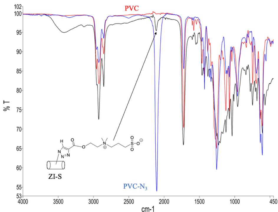
Figure 2.5: Thermal azide-alkyne cycloaddition of an alkyne bearing a zwitterionic group as monitored by ATR-FTIR
