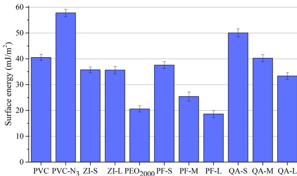
Figure 2.10: Surface free energy of surface modified PVC tubing
