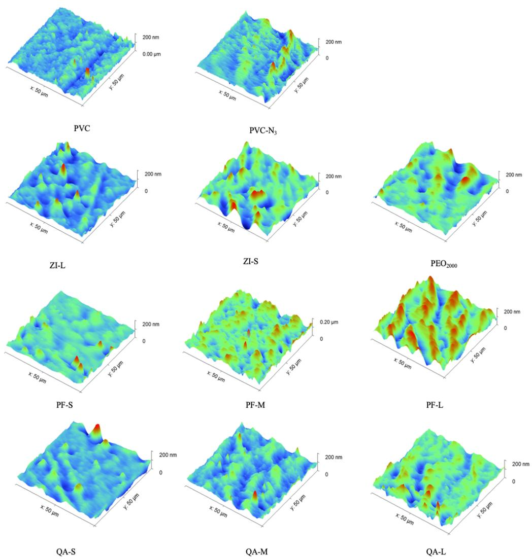
Figure 2.12: AFM images of modified PVC tubing
