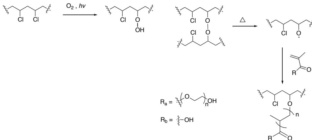
Figure 1.18: PVC surface modification using Gamma-ray with monomers  $R_a$ <sup>73-75</sup> and  $R_b$ <sup>75, 76</sup>
