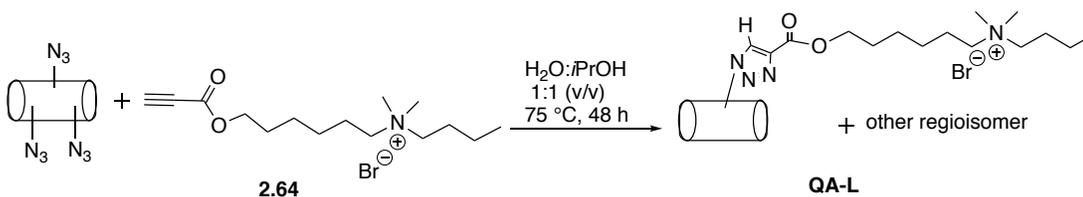
**PVC surface modified by 2-propynoic acid, 5-*N*-butyl-*N*-ethyl-*N,N*-dimethylammonium bromide ester (2.64) (QA-L)**
