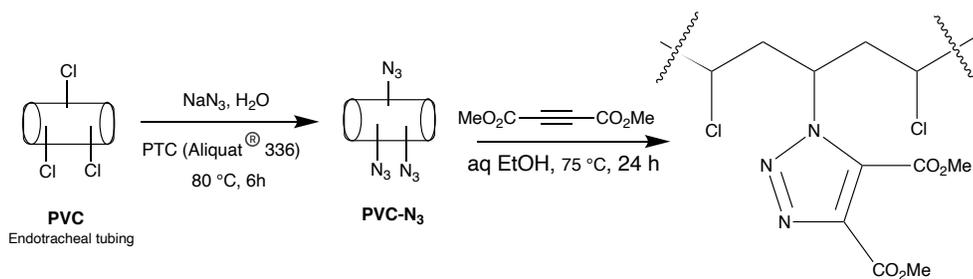
Figure 2.3: Model thermal azide alkyne cycloaddition on azidized PVC tubing
