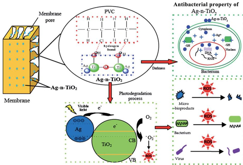
Figure 1.21: Schematic illustration of antifouling properties of Ag-n-TiO<sub>2</sub>/PVC
