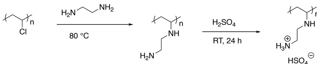
Figure 1.8: Easton's claimed synthesis of sulfonate group-functionalized PVC membrane<sup>51</sup>
