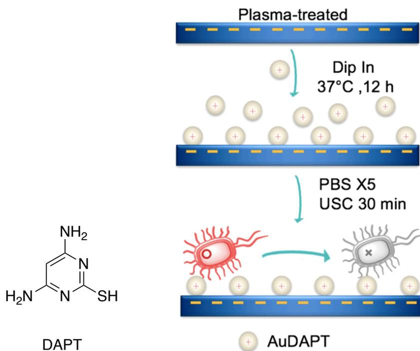
Figure 1.22: AuDAPT based antimicrobial coatings<sup>106</sup>
