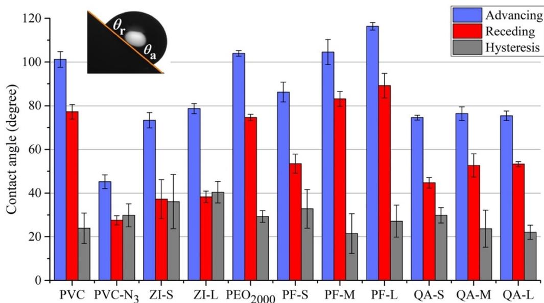
Figure 2.11: Advancing and receding contact angles and contact angle hysteresis (CAH)
