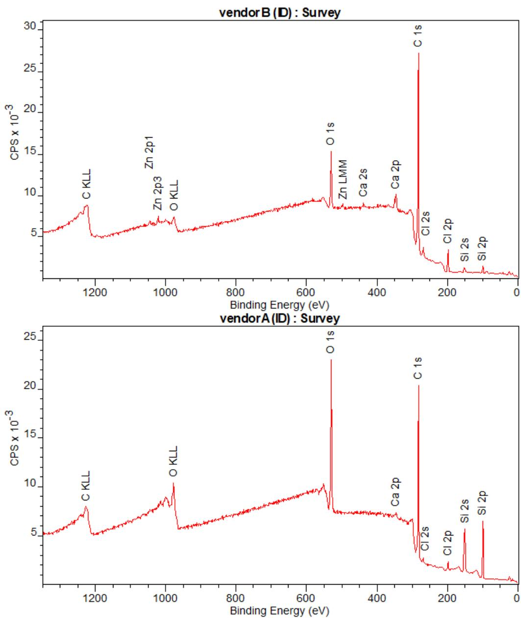
Figure 2.15: XPS of unmodified tubing from vendor B (upper) and vendor A (lower)
