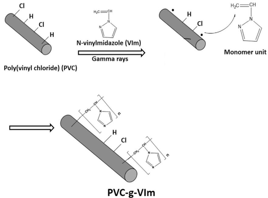
Figure 1.19: PVC surface modification with N-vinylimidazole by gamma ray adopted from reference 77
