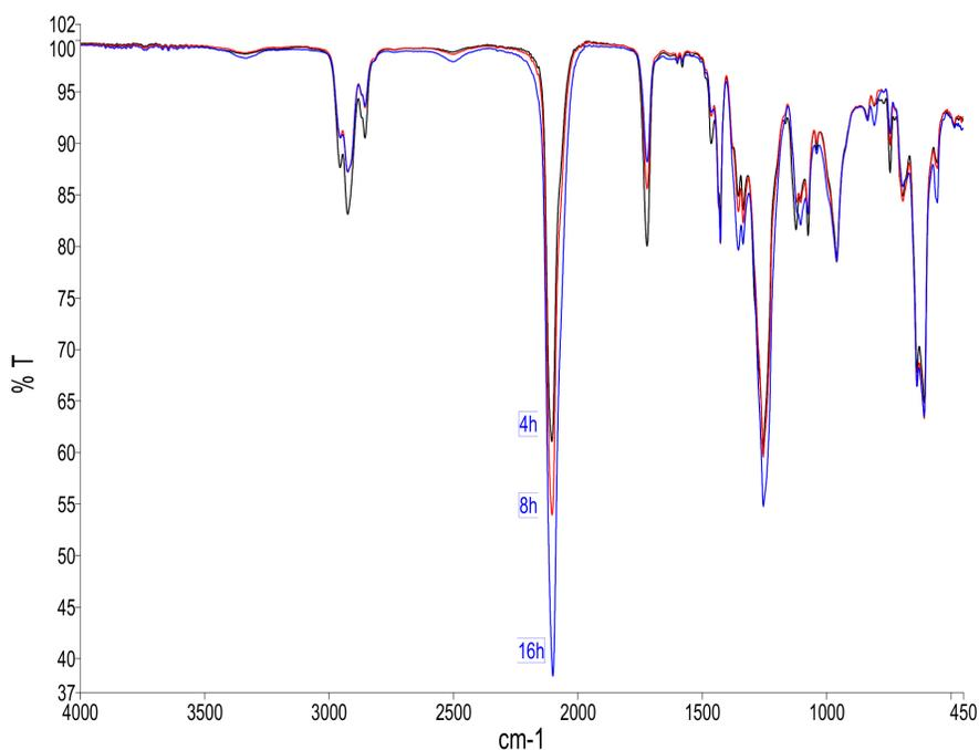
Figure 2.1: Degree of azidation monitored by ATR-FTIR as a function of time: 4, 8 and 16 hours
