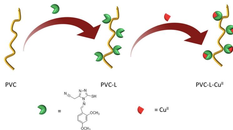
Figure 1.5: Cartoon representation of PVC surface modification by thiol containing a Schiff base, adapted from reference 48
