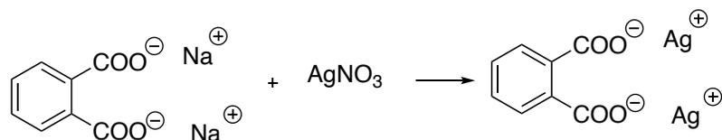
Figure 1.20: Modification of endotracheal tubing by NaOH and  $\text{AgNO}_3$ <sup>92, 93</sup>
