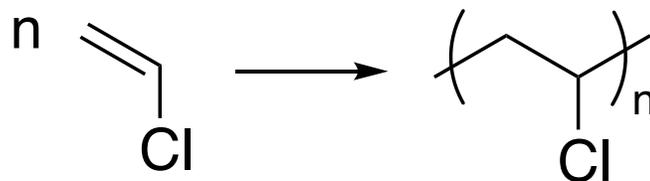
Figure 1.1: Vinyl chloride is polymerized to form PVC
