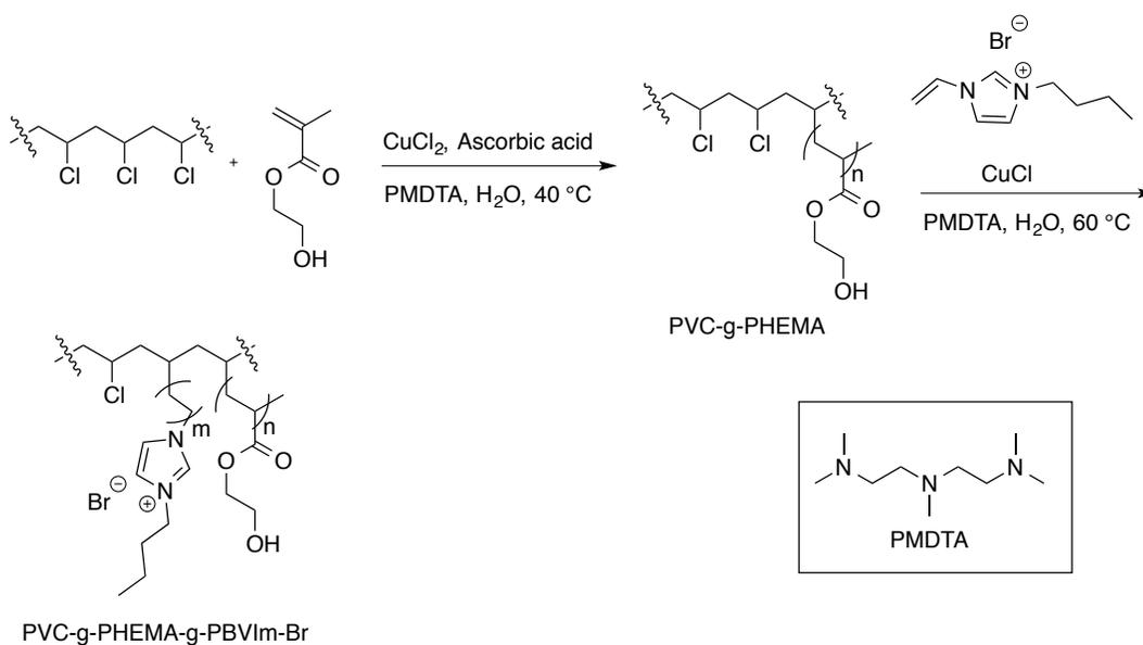
Figure 1.17: Poly(ionic liquid) brushes on PVC membrane using ATRP<sup>68</sup>
