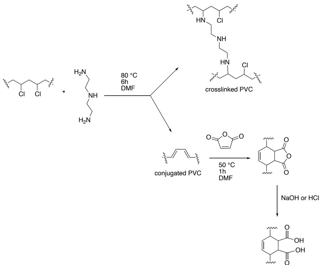
Figure 1.9: PVC modification by multifunctional amines followed by trapping of dienes with maleic anhydride and hydrolysis<sup>52</sup>
