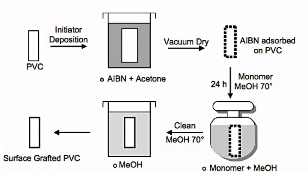
Figure 1.14: Schematic diagram of surface grafting onto PVC adapted from reference
