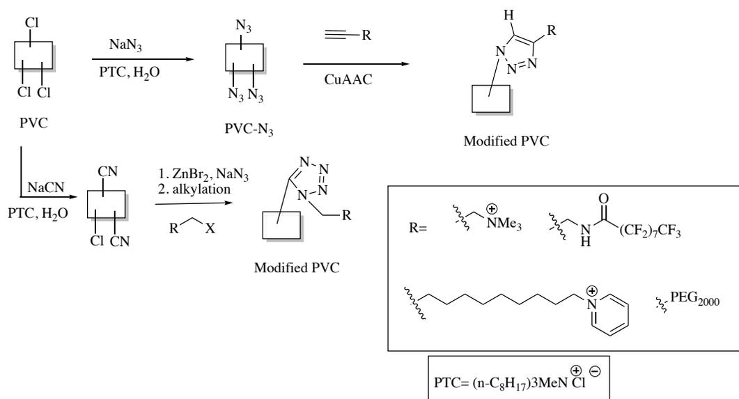
Figure 1.11: Medical grade PVC modification with the CuAAC reaction<sup>61</sup>
