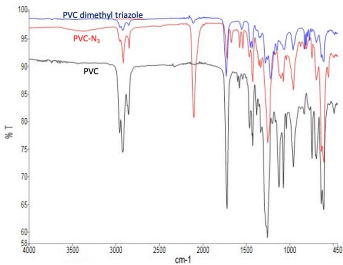
Figure 2.4: Model thermal azide-alkyne cycloaddition on azide functionalized PVC tubing monitored by ATR-FTIR
