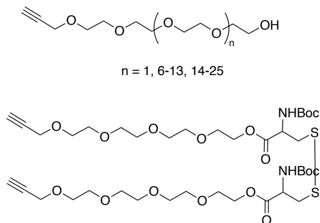
Figure 1.12: Compounds used to modify PVC membrane by CuAAC<sup>62</sup>
