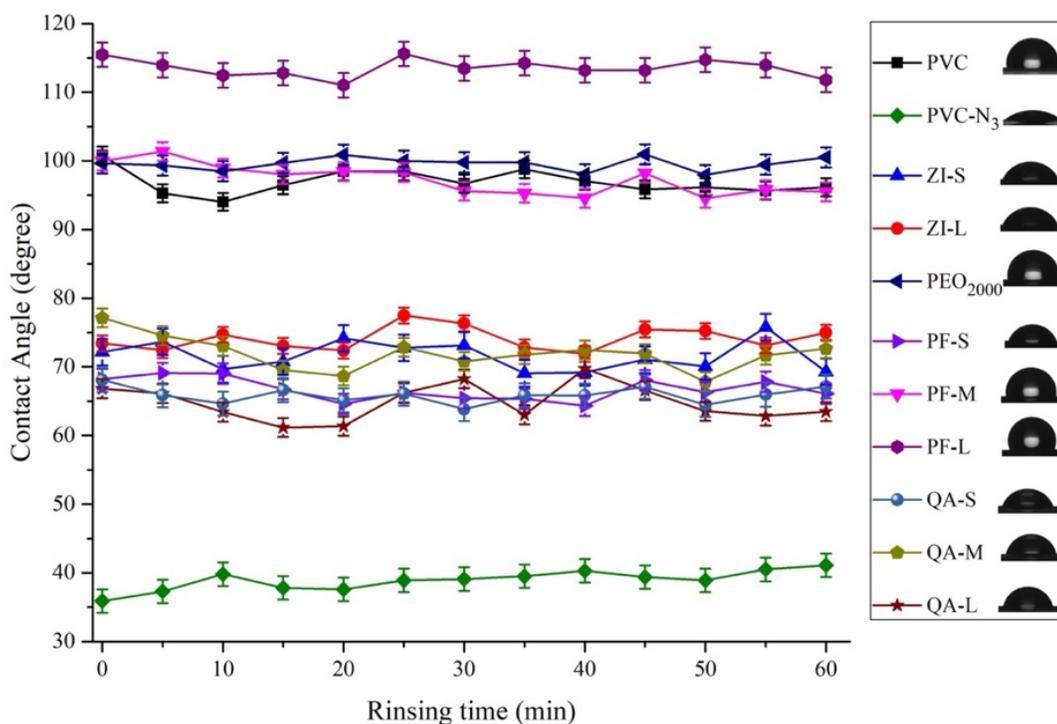
Figure 2.9: Modified PVC surface robustness test
