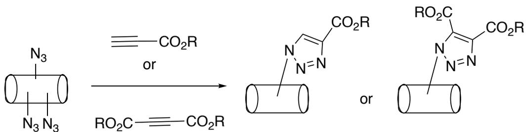
Scheme 1: Thermal azide-alkyne cycloaddition reactions
