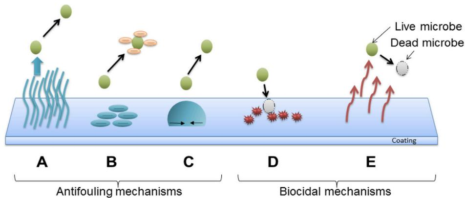
Figure 1.3: Different approaches towards antimicrobial surfaces: A. Surface grafting to create electrostatic repulsion to avoid initial bacterial adhesion. B. Creating charges on coating C. Lowering free energies. D. Biocide release such as silver ions or antibiotics to kill microbials and D. Biocide coating able to kill microbes on contact, adapted from reference 27
