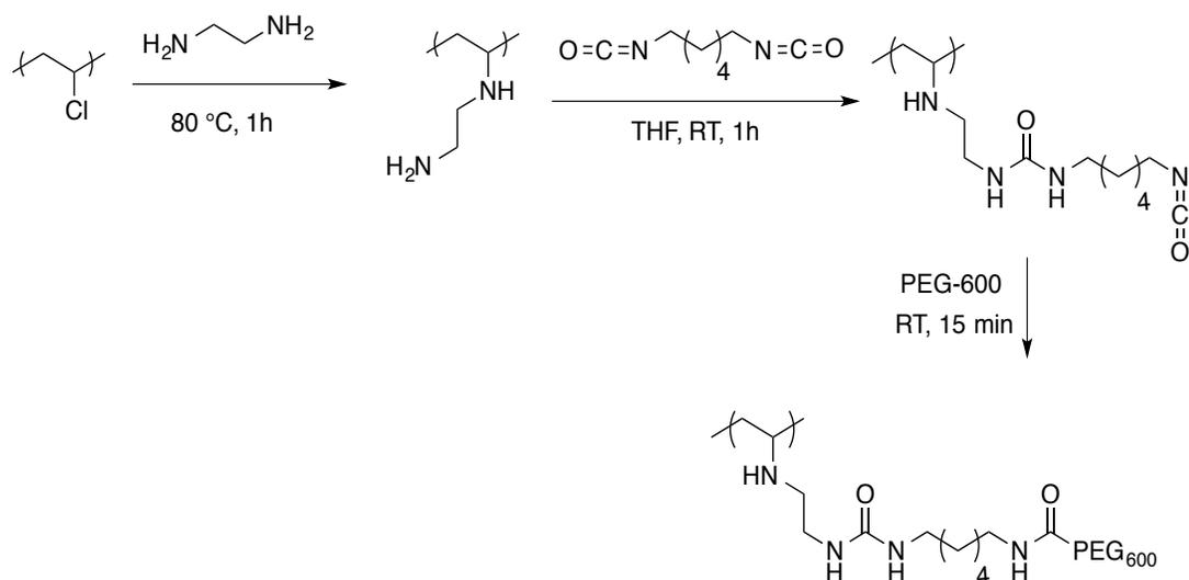
Figure 1.6: Grafting PEG onto PVC<sup>49</sup>
