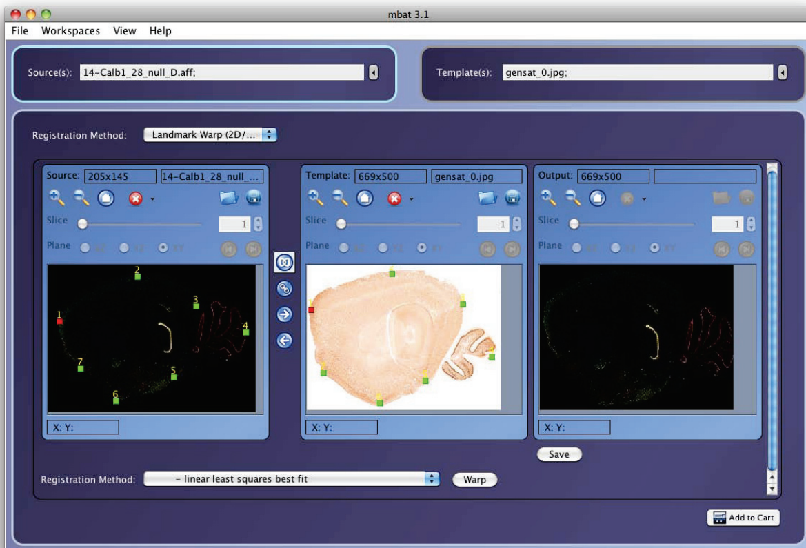
Figure 5 MBAT Registration Workspace Interface. The Registration Workspace showing the results of the LONI Landmark Warp Plug-in. A gene expression image is selected as the source image and shown on the left. The template image is shown in the center, with the paired landmarks overlaid on both the source and template images. The result of the landmark-based registration is shown on the right.
