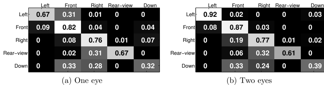
Figure 6.9: Confusion matrix for the five gaze zone classification by participants of de-identified images with (a) one eye and (b) two eyes. Gaze zones are depicted in Figure 6.6. Each row represents true gaze and each column represents the participant's estimate of the gaze zone. Most of the elements in the diagonal have higher percentages than off-diagonal entries. On the average, gaze zone estimation is accurate 65% and 71% for de-identification with one-eye and with two-eyes, respectively.
