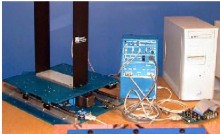
Figure 4. UCIST Shake Table II, power amplifier, personal computer, and test structure, manufactured by Quanser Consulting, Inc.
