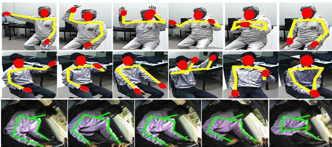
Figure 3.15: Superimposed 3-D pose tracking results on image for visual evaluation. Row 1, 2 - Sample results on a meeting room scene with different test subjects. Row 3 - Sample results on a driving scene.
