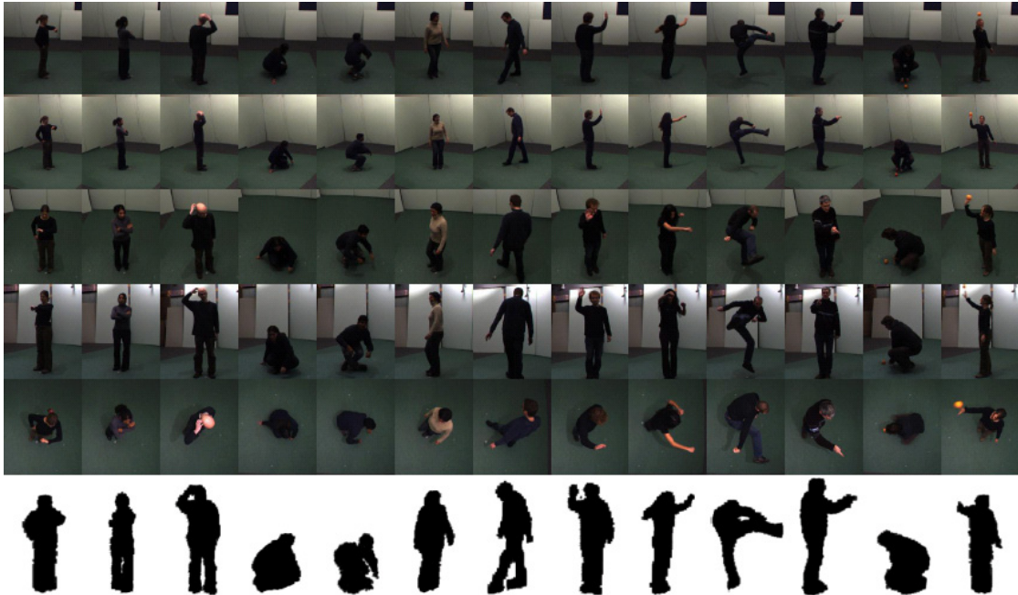
Figure 2.5: Image and 3-D voxel-based volume examples for the 13 actions from the IXMAS Multiview Human Action Dataset. The figure is organized such that the columns correspond to the 13 different actions performed by the 12 actors. The first 5 rows depict images captured from the 5 camera views, while the 6 th row shows the corresponding 3-D volumes.
