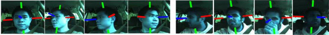
Figure 4.8: Visual evaluation of HyHOPE head pose tracking with large range of head rotation, change in lighting condition, and some occlusions.
