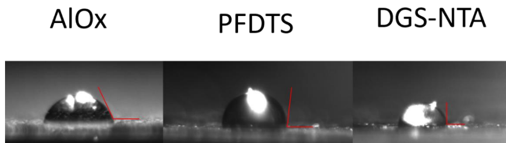
Figure 4. Water droplet contact angle comparisons to confirm the hydrophobicity of the surface.
