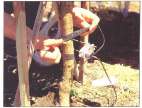
Attachment strap on mounting bracket of linear variable displacement transducer (LVDT) is affixed to the tree trunk.
