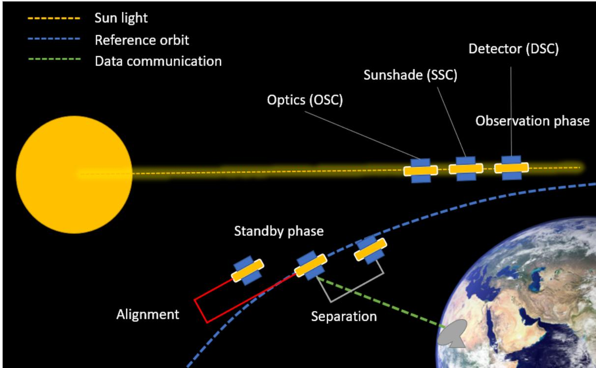
**Figure 2.1:** VISORS mission phases and 3U CubeSats formation flying.
