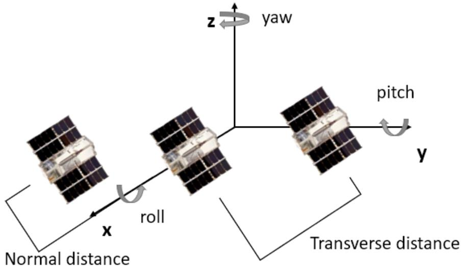
**Figure 4.2:** CubeSat attitude alignment and separation
