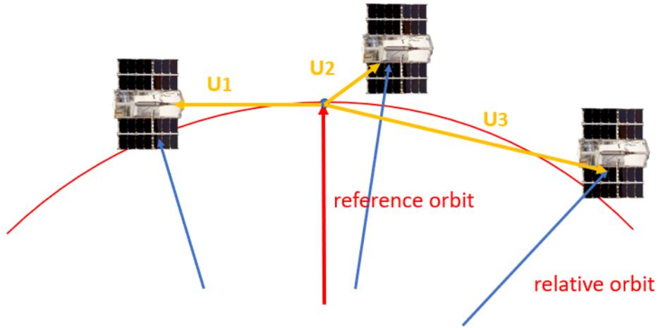
**Figure 4.1:** Reference orbit and relative orbits of three Cubesats
