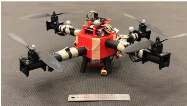
Figure 26. Tilting Multicopter rotors for Increased Power Efficiency and Yaw Authority
