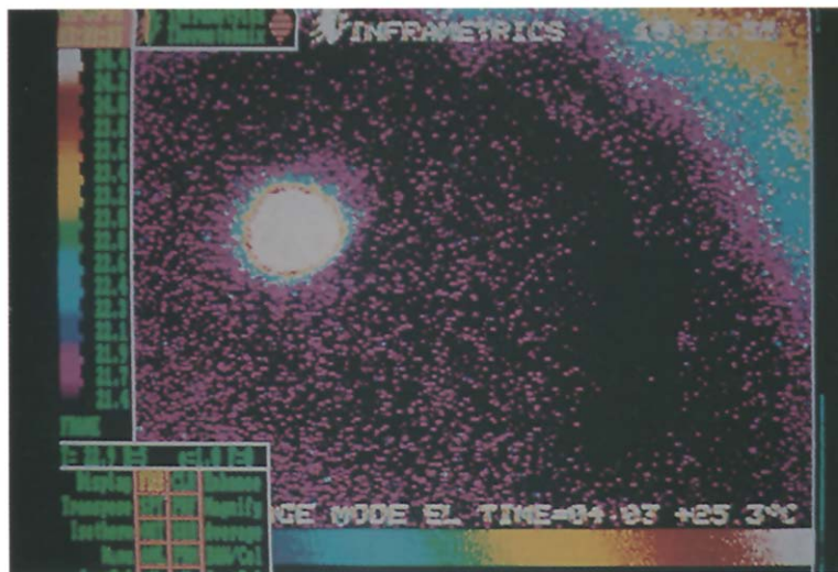
Fig. 2. The temporal bone illustrated here was treated with a CO 2 laser at 4 W power and a 200 \mu m focused spot size. This image was obtained at the end of a 100 msec laser pulse.
