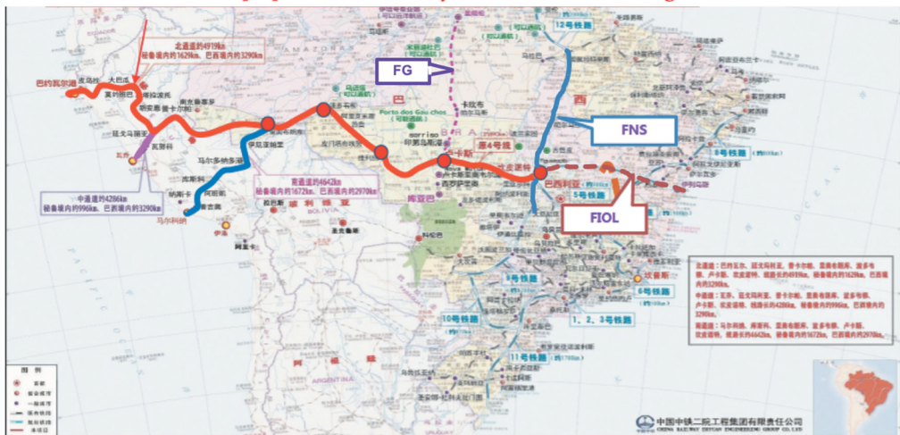
Proposed nodes for Bi-Oceanic Railroad in red, with three alternative routes for the western terminus in Peru, no defined eastern terminus in Brazil, and connections with the recently build North-South Railroad (FNS), and the proposed Grain Railway (FG) and West-East Integration Railroad (FIOL).
