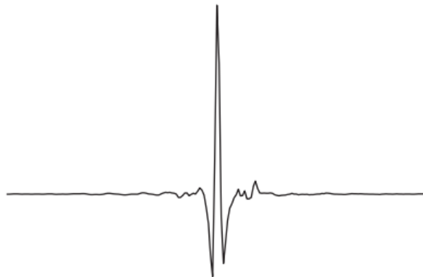
Fig. 6.5 Typical interferogram of the broadband light source in the region of the centerburst.
