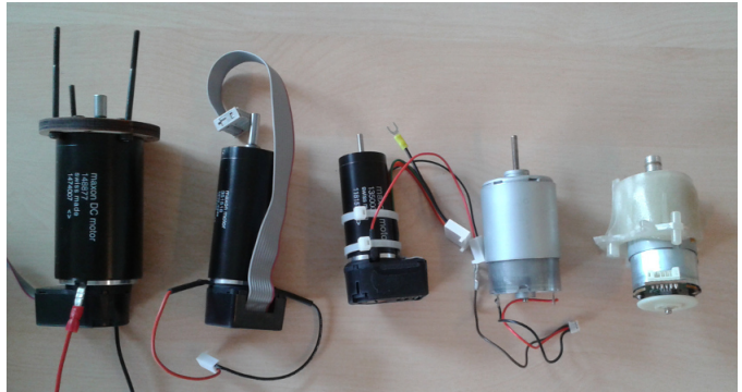
Fig. 9. Different motors that have been used for haptic devices, from left: Maxon RE40, Maxon RE30, Maxon RE25 (Phantom), Mabuchi RS-555PH (Falcon), Mabuchi RS-455PA (Omni)
