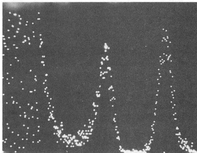
Figure 8. Measured radiation spectrum for a 1.4 mm 2 detector with on-chip amplifier. The shaper time constant was 200 ns. The lower peak is the 60 keV gamma ray from an Am 241 radiation source, and the upper peak is a voltage pulser set to inject 4 fC. The FWHM is \approx 6.8 keV, equivalent to an input noise charge of 800 electrons r.m.s. The lower photograph shows an expanded view.
