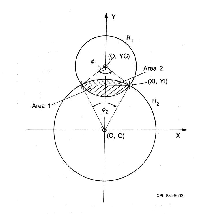
Fig. 2 Diagram in plane of larger counter showing how the overlap area is calculated from the sum of two segments, one from each circle.
