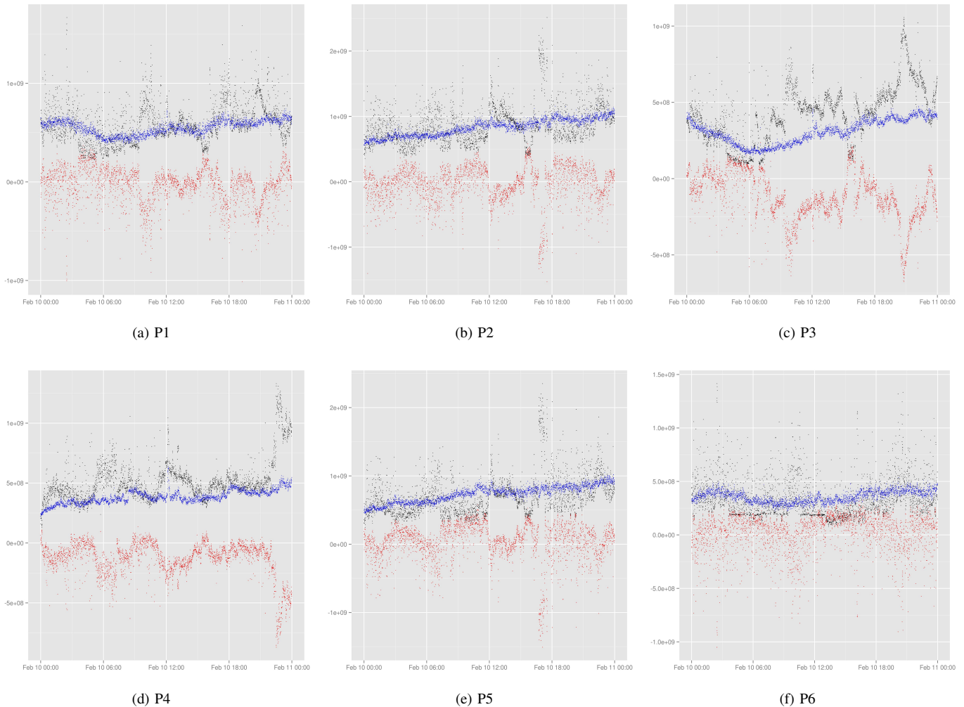
Fig. 11: Bandwidth Utilization Forecast: The forecast is for one target date, Feb. 10, GMT 2014. Black colors are for the observed data. Blue colors are for the forecasts. Red colors are for the forecast errors.
