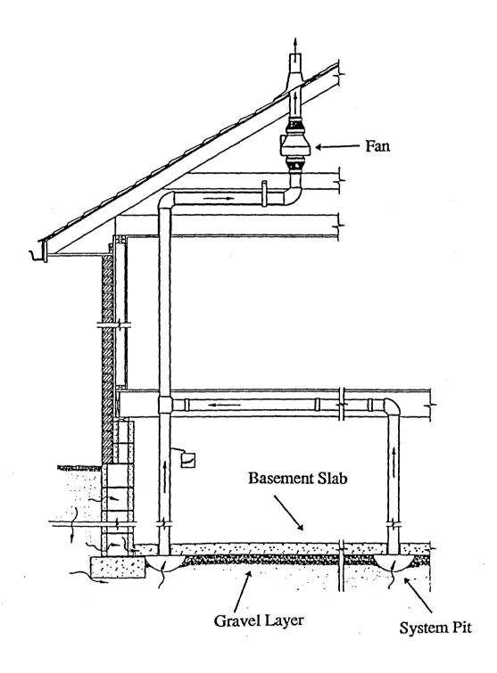
Figure 1. Schematic of an SSD system [38]. The system fan draws radon-bearing soil gas from the pit and exhausts it to the outdoors.
