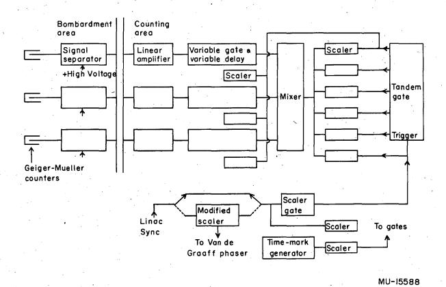
Fig. 7. Block diagram of electronic circuitry.
