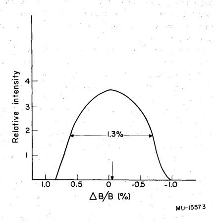
Fig. 11. Resolution function of the spiral-orbit-spectrometer for a 1/8-in. beam and a conical target. The arrow indicates the position of the ordinate bisecting the area under the curve.
