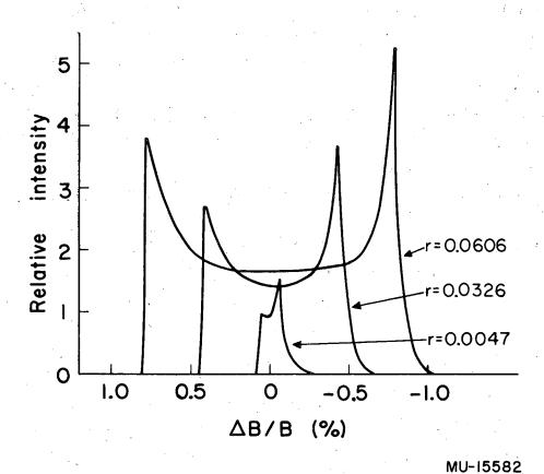
Fig. 20. Spectrometer resolution for cylindrical shells weighted by their radii. The "0" corresponds to the energy or momentum of a particle in the focal orbit. The probability of focusing higher-energy particles is represented by the right side of the curves.
