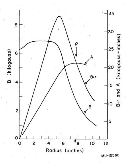
Fig. 4. Radial distribution of the magnetic field, vector potential, and B·r corresponding to 15.6 Mev. The intersection of A and B·r determines  $\rho$ .
