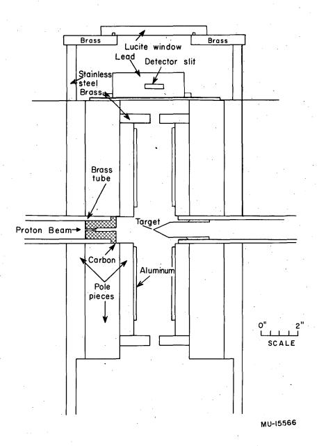
Fig. 2. Cross section through spectrometer. The pole tips, target, slits, detector, and vacuum chamber are shown.
