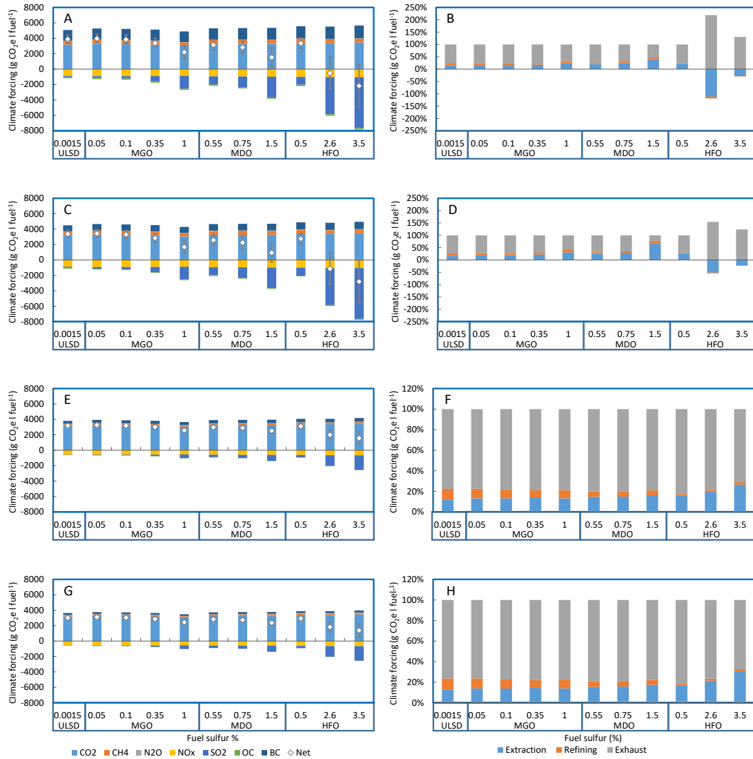
Figure 2.6: Total fuel-cycle (crude oil extraction, crude refining, and vessel fuel-exhaust emission) climate forcing of marine fuels by chemical constituent, marine fuel type, and engine characteristics on 20-y and 100-y time horizons. The marine fuels include distillates and heavy fuel oil (HFO). The distillates include ultra-low sulfur diesel (ULSD), marine gas oil (MGO), and marine diesel oil (MDO). The chemical constituents include black carbon (BC), organic carbon (OC), sulfur dioxide (SO 2 ), nitrogen oxides (NO x ), nitrous oxide (N 2 O), methane (CH 4 ), and carbon dioxide (CO 2 ). The engine characteristics include medium-speed diesel (MSD) and high-speed diesel (HSD) engines. Left panels (A,C): total fuel-cycle climate forcing by chemical constituent. Right panels (B,D): mean percent (%) contribution of each phase to the total fuel-cycle climate forcing. First and third rows (A,B,E,F): total-fuel climate forcing of MSD engines. Second and fourth rows (C,D,G,H): total fuel-cycle climate forcing of HSD engines. First and second rows (A,B,C,D): 20-y time horizon. Third and fourth rows (E,F,G,H): 100-y time horizon. The error bars represent the 95% confidence interval.
