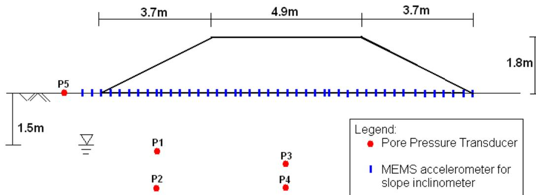
**Fig. 1. Schematic of test levee with sensors used in long-term remote measurements.**
