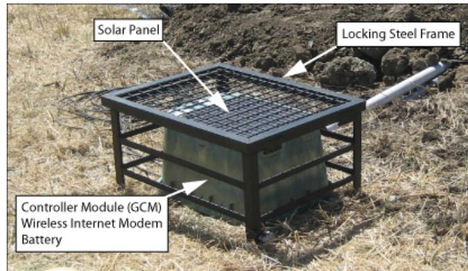
**Fig. 4. Remote monitoring station.**
