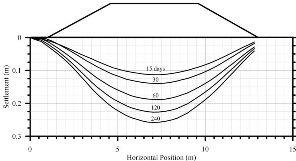
**Fig. 7. Settlement profiles at various times following construction of the model levee.**
