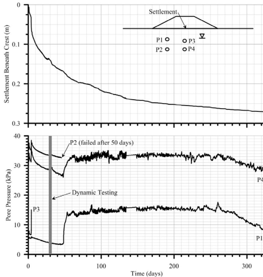
**Fig. 6. Settlement beneath levee crest and pore pressure at various positions beneath the embankment versus time for 325 days.**
