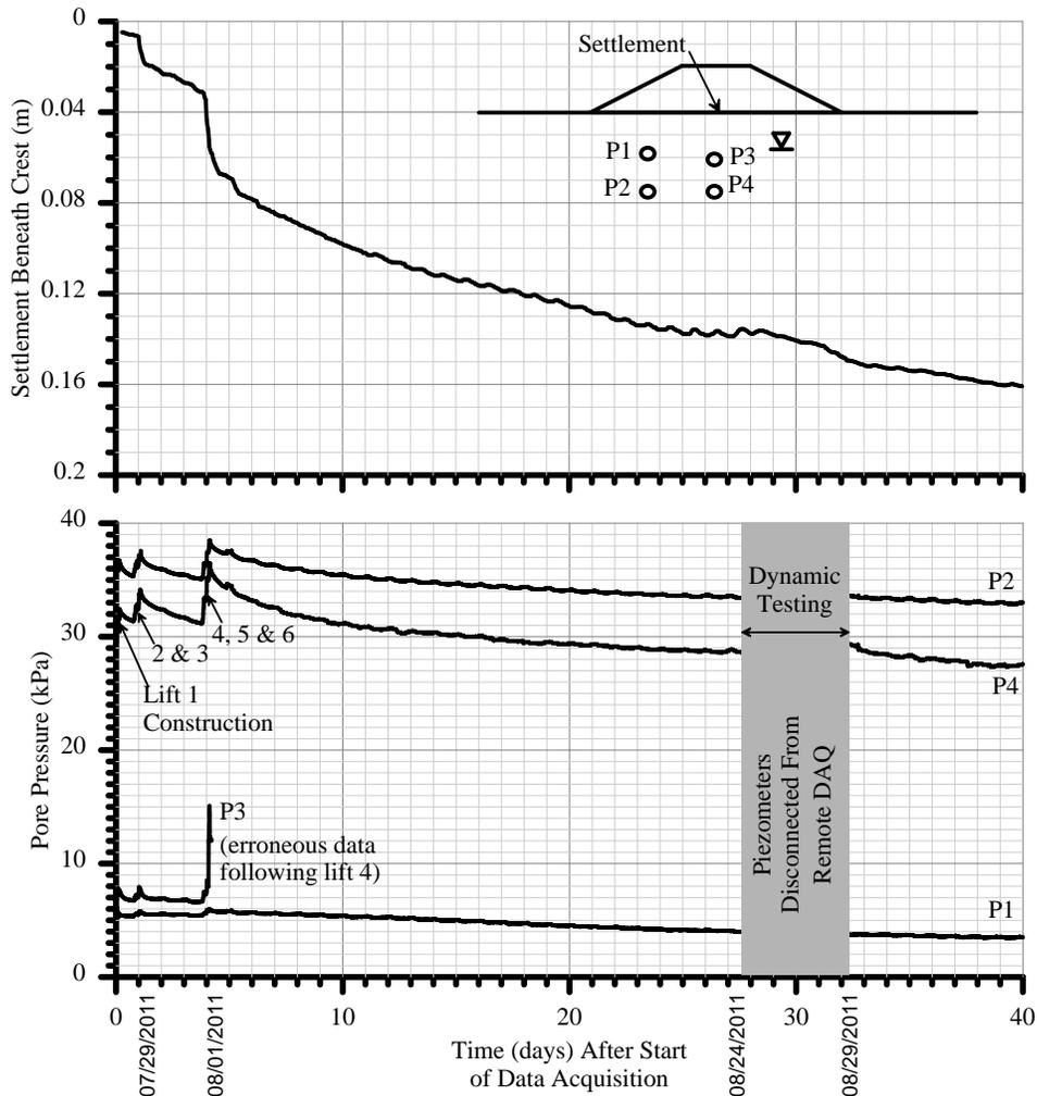
**Fig. 5. Settlement beneath levee crest and pore pressure at various positions beneath the embankment versus time for 40 days following embankment construction, including the period following dynamic testing.**
