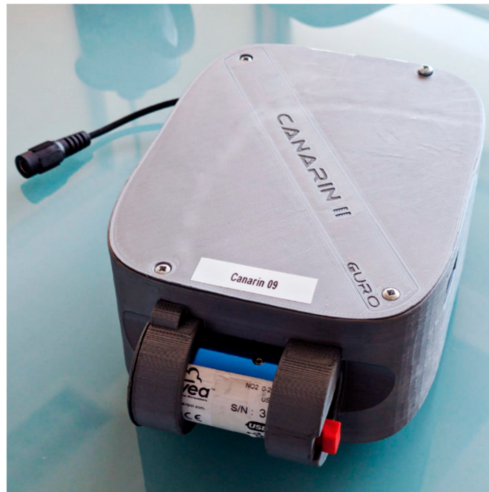
Figure 2. Canarin II in grey. The Cairsens NO 2 is conveniently attached to it.
