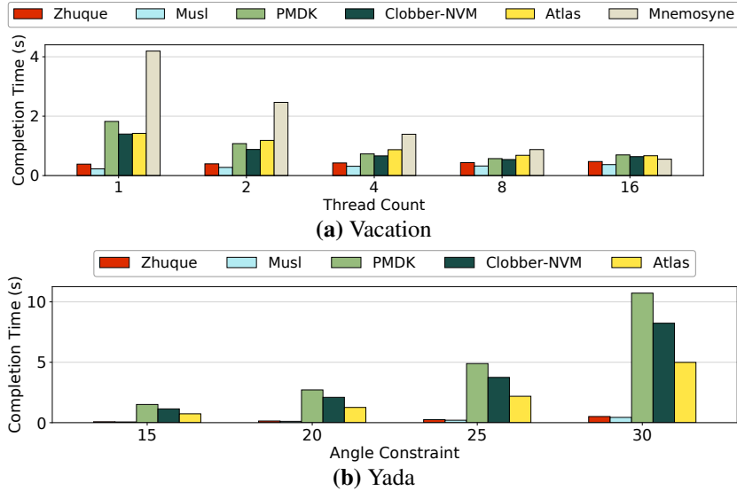
Figure 4.9. Vacation and Yada performance on different PMEM libraries and Zhuque. Zhuque outperforms Mnemosyne, PMDK, Atlas and Clobber-NVM, respectively. The performance gain comes from fewer logging writes and more efficient memory management: Zhuque uses vanilla malloc() , while the other libraries use either PMDK’s transactional allocator (PMDK, Clobber-NVM) or a hand-written allocator (Mnemosyne, Atlas). The memory management efficiency problem is more prominent on Yada, which implements Ruppert’s algorithm for Delaunay mesh refinement [101].
