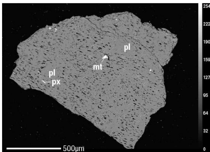
**Fig. 2.** BSE image of sparsely phyric rhyolite melt encountered at approximately 2100 m depth in IDDP-1 well and quenched to glass by drilling fluid. The high silica rhyolite (Table 1) is poorly vesiculated with phenocrysts of plagioclase (pl), pigeonite and augite (px), and titanomagnetite (mt).
