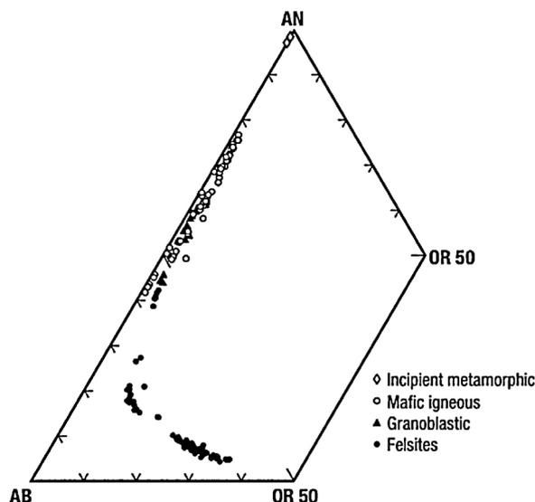
Fig. 5. Composition of feldspars from mafic and felsic rock cuttings recovered from IDDP-1.
