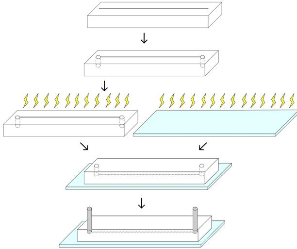
Figure A.2: PDMS fabrication and irreversible bonding.
