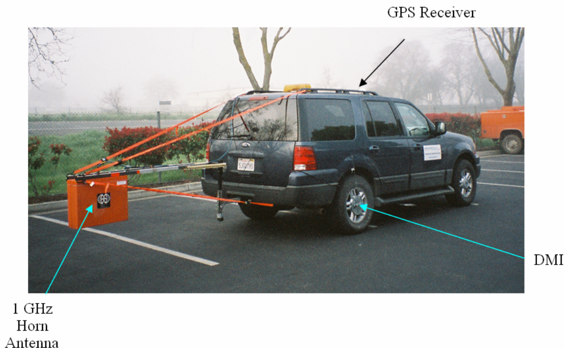
Figure 4. GPR equipment used on this project.
