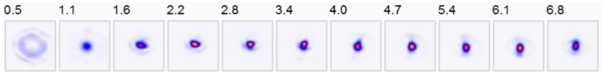
(b) Image size 1019 \mu\text{m} . Red beam at capillary exit, 70 mm iris. Fluences are for values of n_{\text{H}_2} in units of 1 \times 10^{17} \text{ cm}^{-3} .
