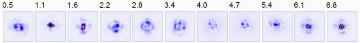
(a) Image size 1019 \mu\text{m} . Red beam at capillary exit, 125 mm iris. Fluences are for values of n_{\text{H}_2} in units of 1 \times 10^{17} \text{ cm}^{-3} . Saturation in some images is due to color scale bounds set to emphasize low signal regions.
